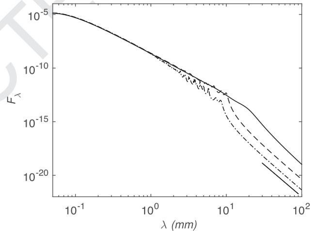
**Figure 6.** Smoothed and averaged SEDs for compacted grains consisting of a silicate matrix with inclusions of FeS occupying volume fractions of  $f = 0$  (lower curve, dot-dashed line),  $f = 0.1$  (middle curve, dashed line, as shown in Fig. 5) and  $f = 0.3$  (upper curve, solid line). The slope bar in the lower right-hand side indicates an exponent of  $-6$ .
