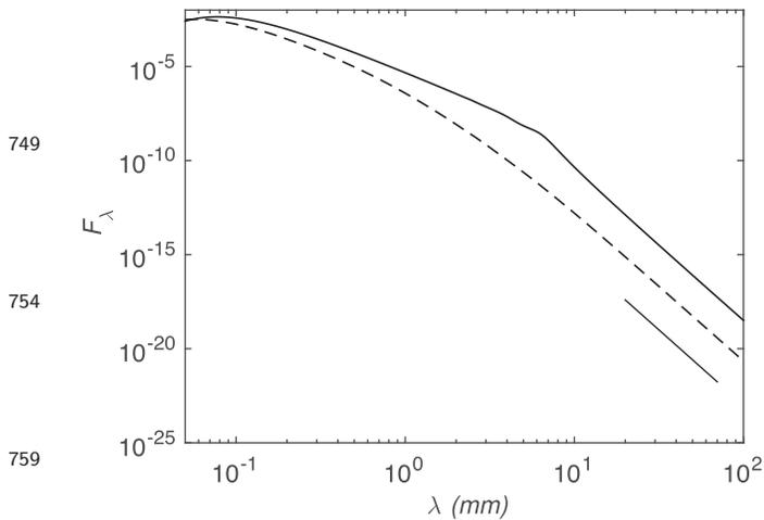
**Figure 7.** SEDs for clustered aggregates consisting of FeS monomers with no silicate, occupying volume fractions of  $f = 0.1$  (lower curve, dashed line) and  $f = 0.3$  (upper curve, solid line). The slope bar in the lower right indicates an exponent of  $-8$ .
