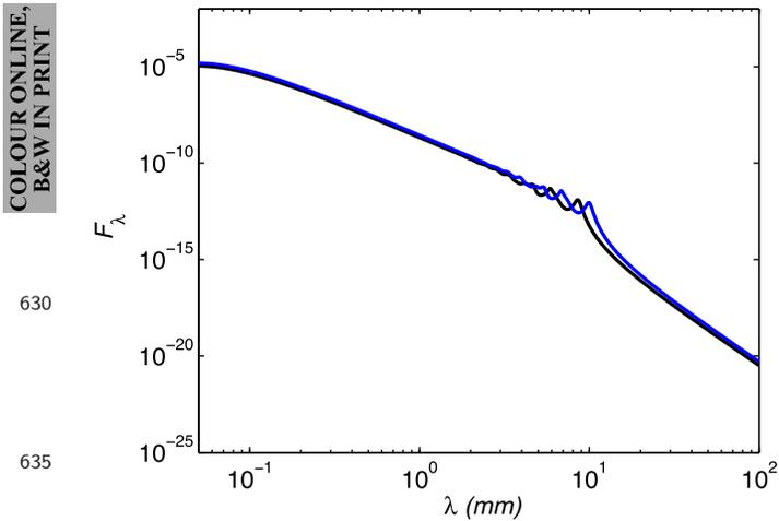
**Figure 4.** SEDs for compacted grains consisting of a silicate matrix with inclusions of FeS occupying a volume fraction  $f = 0.1$ . Results for two different grain sizes are shown: radii 1 (black) and 1.16 mm (blue).
