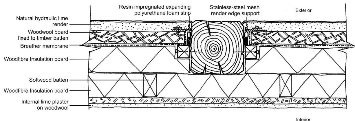
Figure 6 Replacement panel infill detail with internal lining. Source: (Author's own based on (Demaus, 2015) adaptation of Historic England detail (McCaig and Ridout, 2012))
