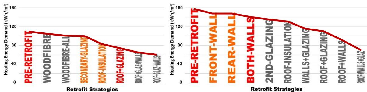
Figure 10. Simulated Heating Energy Demand (kWh/m<sup>2</sup>) for The Oaks (left) and The Old Mayor's Parlour (right) Hypothetical scenarios in grey, individual retrofit actions in orange and as-built in red
