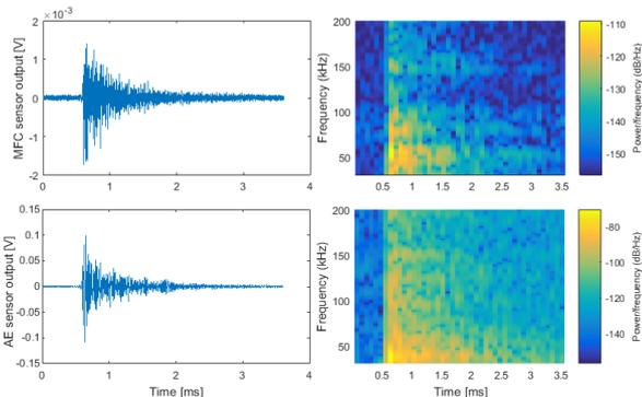
**Figure 1:** (a) design of the patch and experimental setup; (b) waveforms from MFC sensor (top) and legacy AE sensor (below), and their spectrograms (right).
