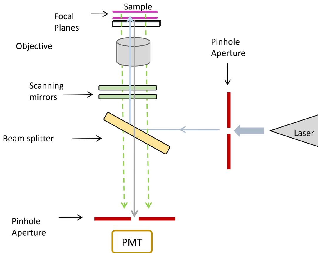
**Figure 2.2 Schematic of confocal imaging system using an inverted microscope**
