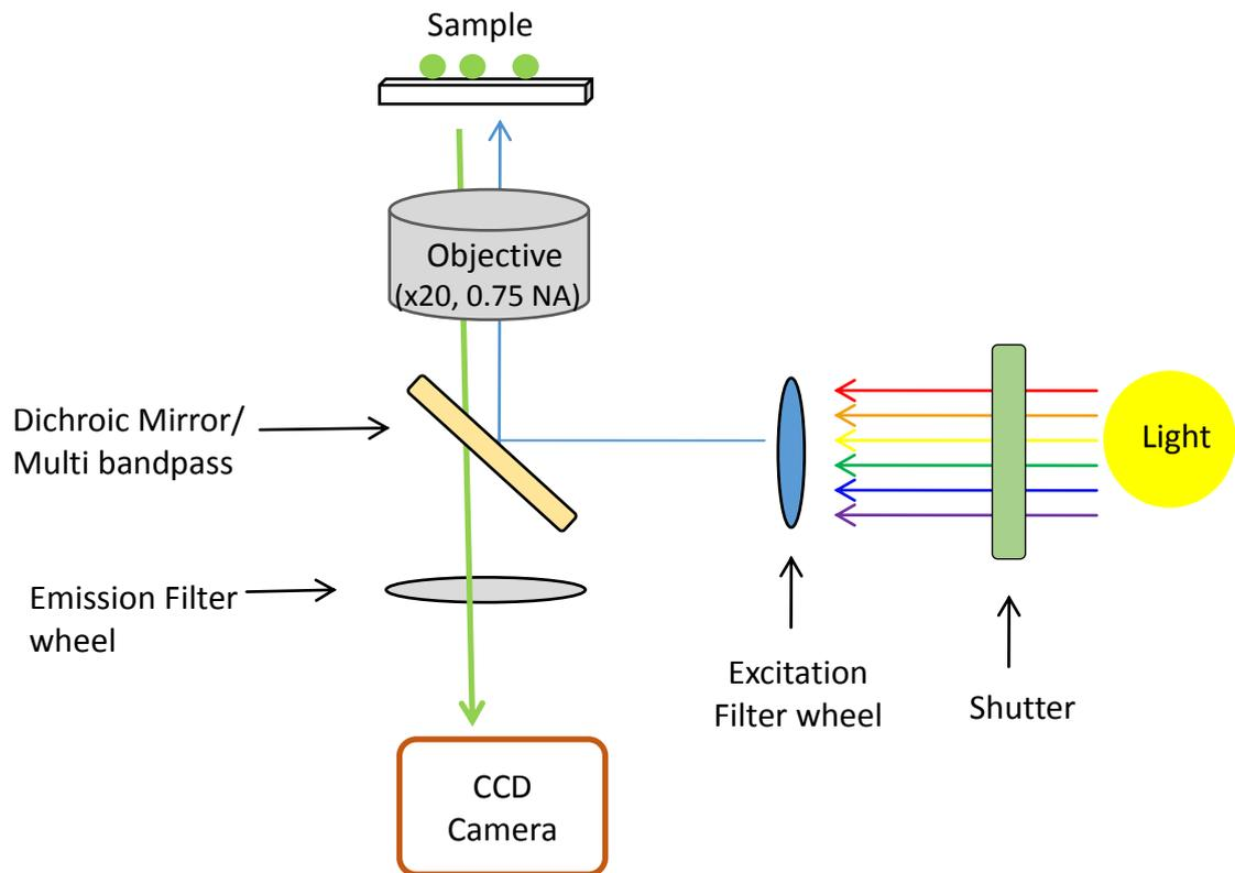
**Figure 2.1 Schematic of epifluorescence imaging system using an inverted microscope**
