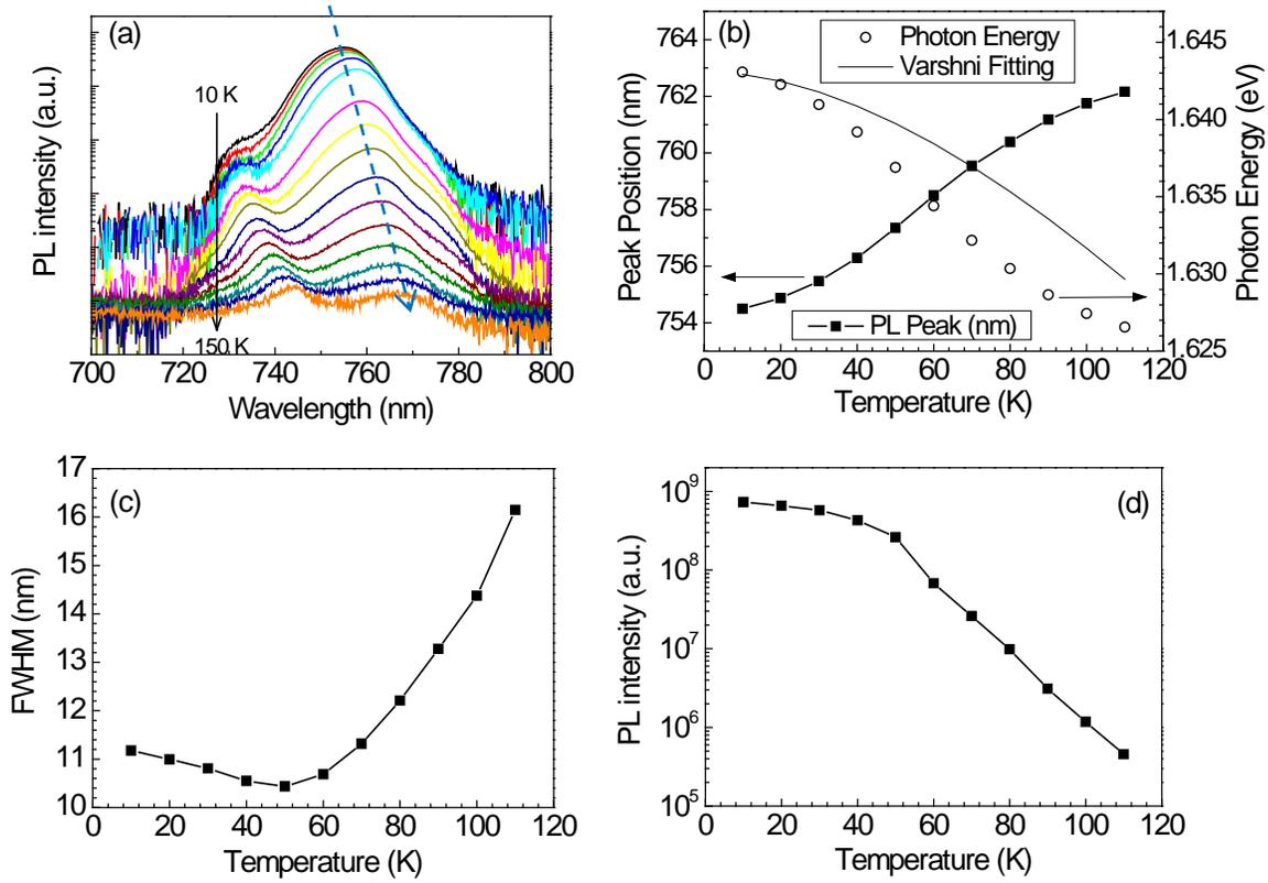
Figure 5. (a) Temperature-dependent PL spectra of GaAs/Al<sub>0.2</sub>Ga<sub>0.8</sub>As hybrid nanostructures measured at an excitation laser intensity of 3000 W/cm<sup>2</sup>; The peak position (b), FWHM (c), and integrated intensity (d) of the wetting ring peak are extracted as a function of the temperature
