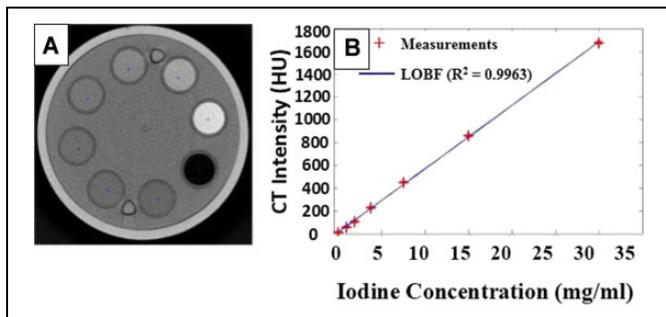
**Figure 5.** A, Reconstructed image of the Shelley microCT phantom with 8 different concentrations of iodine. B, CT number (HU) measurements and a line of best fit (LOBF) plot for different concentrations of iodine (range: 0-30 mg/ml) was linear. CT indicates computed tomography; HU, Hounsfield unit.
