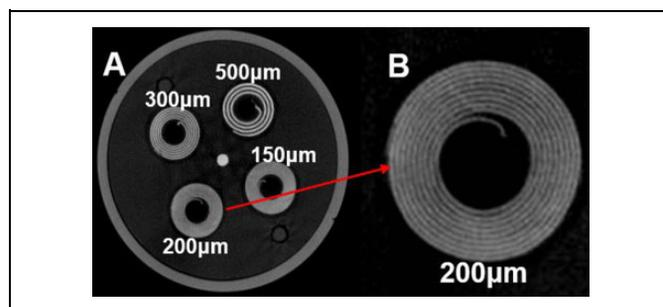
**Figure 3.** (A) SACRTD reconstructed axial image of the resolution coil plate in the Shelley microCT phantom and (B) magnified view of the smallest coil that can be resolved by naked eye ( $200 \mu\text{m}$  layer thick coil corresponding to 2.5 lp/mm). SACRTD indicates small animal conformal radiation therapy device.
