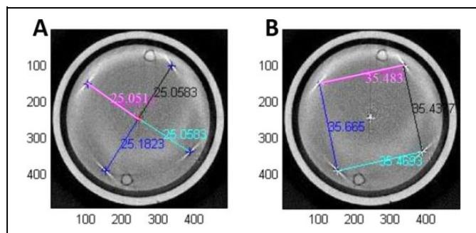
**Figure 2.** SACRTD reconstructed image of the Shelley microCT QA phantom showing geometric distance between the (A) 4 corner beads from the center bead and (B) 4 corner beads from one another. The measurements were within 2% of the manufacturer specified distances of 24.75 and 35 mm, respectively. CT indicates computed tomography; SACRTD, small animal conformal radiation therapy device.
