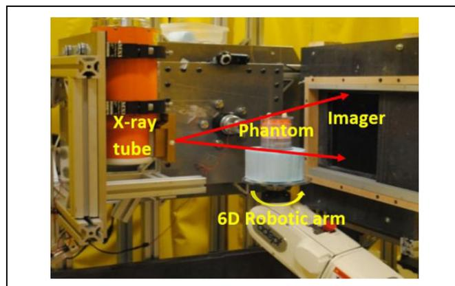
**Figure 1.** Cone beam CT acquisition configuration of SACRTD with static gantry and a micro CT imaging phantom rotating on the palm of the robotic arm. CT indicates computed tomography; SACRTD, small animal conformal radiation therapy device.
