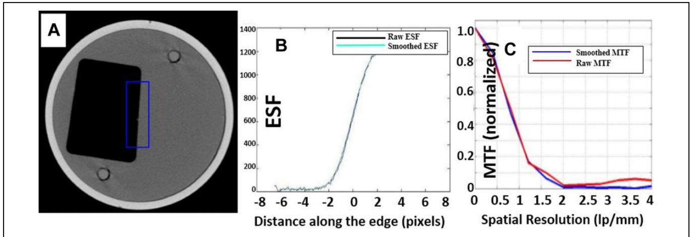
**Figure 4.** A, Axial reconstructed image of the Shelley microCT phantom with slant edge showing region of interface with air. B, ESF—raw and Gaussian smoothed as a function of distance across the edge. C, Raw and Gaussian smoothed MTF variation with spatial resolution (lp/mm). CT indicates computed tomography; ESF, edge spread function; MTF, modulation transfer function.
