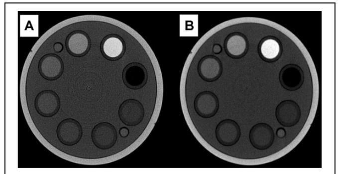
**Figure 6.** (A) Reconstructed axial slice of the CT linearity plate in the Shelley microCT phantom with ring artifacts and (B) the corresponding median filtered image. CT indicates computed tomography.
