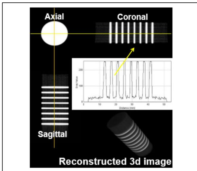
**Figure 9.** Axial, coronal, and sagittal slices of the QRM microCT Multidisk phantom with overlay of the profile along longitudinal direction and the reconstructed 3-dimensional images. CT indicates computed tomography.
