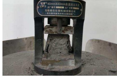
Figure 2. Compressive strength testing
