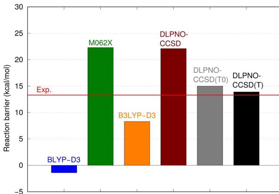
**Figure 1** QM/MM reaction barriers for the hydroxylation reaction in the active site of PHBH at various level of QM theory. The results are obtained by averaging the values obtained from 10 different snapshots (see Tables 1 and 2). The horizontal red line marks the available experimental value.
