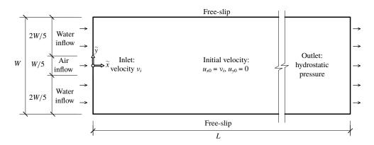
FIGURE 5. The 2-D model set-up for numerical simulation.
