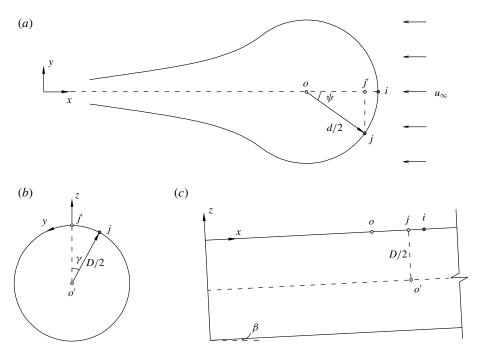
FIGURE 14. (a) The unrolled geometry of a bubble in the x-y plane, and the views of (b) a transversal cross-section in the y-z plane and (c) a longitudinal cross-section in the x-z plane.
