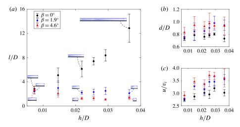
FIGURE 11. (Colour online) Variation of bubble properties with the gap thickness h while the pipe diameter D is fixed to be 0.137 m: (a) normalised bubble length l/D, (b) normalised bubble cap diameter d/D and (c) normalised bubble terminal velocity  $u/v_i$ .
