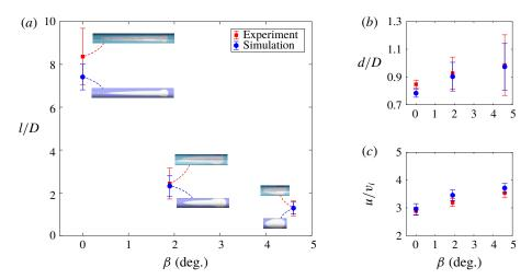
FIGURE 10. (Colour online) Variation of bubble properties with the inclination angle  $\beta$ : (a) normalised bubble length l/D, (b) normalised bubble cap diameter d/D and (c) normalised bubble terminal velocity  $u/v_i$ .
