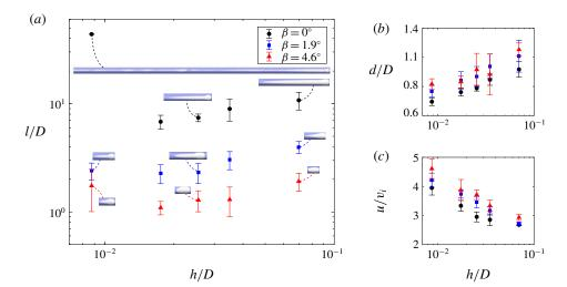
FIGURE 12. (Colour online) Variation of bubble properties with the pipe diameter D while the gap thickness h is fixed to be 0.0035 m: (a) normalised bubble length l/D, (b) normalised bubble cap diameter d/D and (c) normalised bubble terminal velocity  $u/v_i$ .
