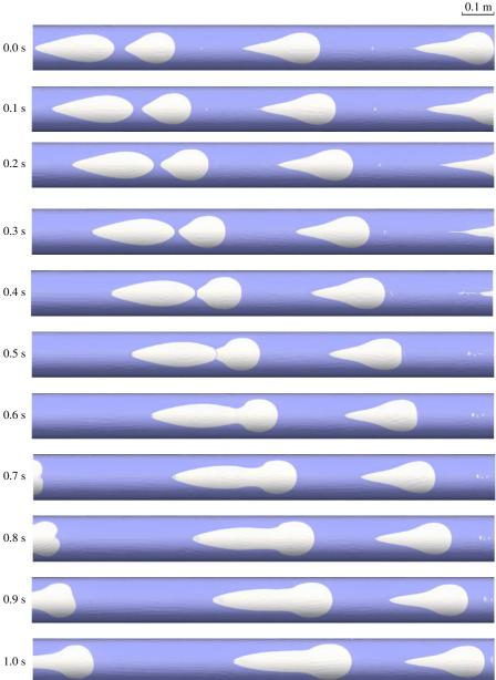
FIGURE 8. (Colour online) Simulation results showing the coalescence process for two bubbles in the 1.9° inclined annulus.
