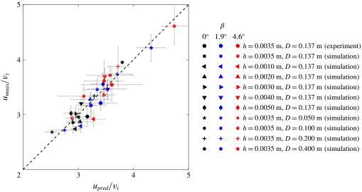
FIGURE 15. (Colour online) Comparison of the predicted terminal velocity  $u_{pred}$  from (5.5) and the measured terminal velocity  $u_{meas}$  from experiments and simulations for different configurations of pipe diameter D, gap thickness h and inclination angle  $\beta$ . The velocity values are normalised by the superficial inflow velocity  $v_i$ .
