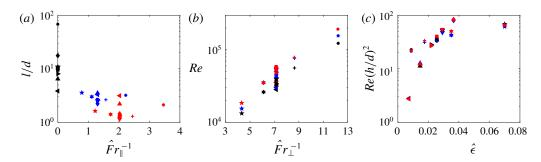
FIGURE 16. (Colour online) (a) Variation of the bubble aspect ratio l/d with the inverse Froude number  $\hat{F}r_{\parallel}^{-1}$ . (b) Variation of the bubble Reynolds number Re with the inverse Froude number  $\hat{F}r_{\perp}^{-1}$ . (c) Variation of the gap Reynolds number  $Re(h/d)^2$  with the confinement ratio  $\hat{\epsilon}$ . Refer to figure 15 for the legend.
