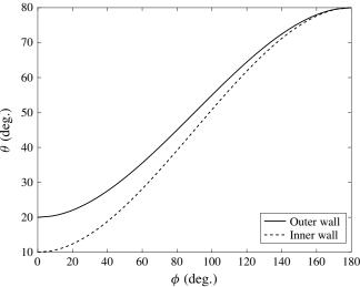
FIGURE 4. Interpolation of contact angles around a contact line at the outer or inner wall of the annulus using a third-order polynomial fitting (Antonini *et al.* 2009);  $\theta$  denotes the local contact angle and  $\phi$  denotes the intersection angle between the local velocity vector and the interface normal as shown in figure 3.
