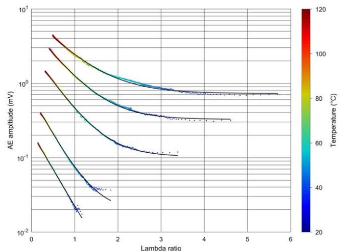
**Figure 1:** Band-passed AE signals collected at five different fast disk operating speeds (from bottom, 300, 500, 1000, 1500, 2000 rpm), shown as a function of specific film thickness
