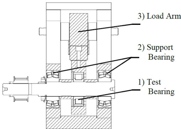
**Figure 2:** Schematic of bearing rig test head
