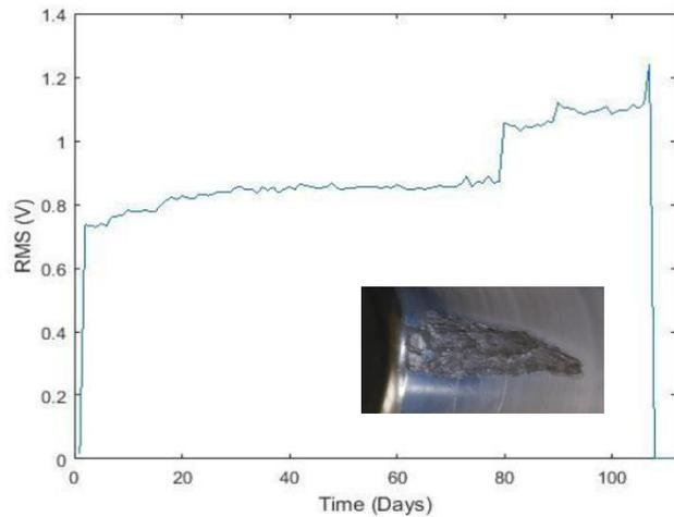
**Figure 3:** RMS AE levels during bearing life test
