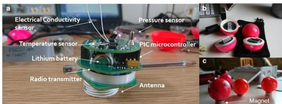
**Fig. 2.** ET+ platform design, showing the triple stacked circuit boards with sensors and antenna (a), which is later potted into two half-spheres (b) and fixed together with resin prior to deployment (c). Note the magnets in (c) used to switch off the assembled ET+ via a reed switch.
