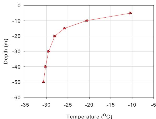
**Fig. 5.** Temperature transmitted by the ET+, received by the ApRES, during a 60 m borehole log. The sensor remained at each depth for  $\sim 5$  min, and the plotted temperature is the data point transmitted at the end of this period, after the sensor was allowed to equilibrate.
