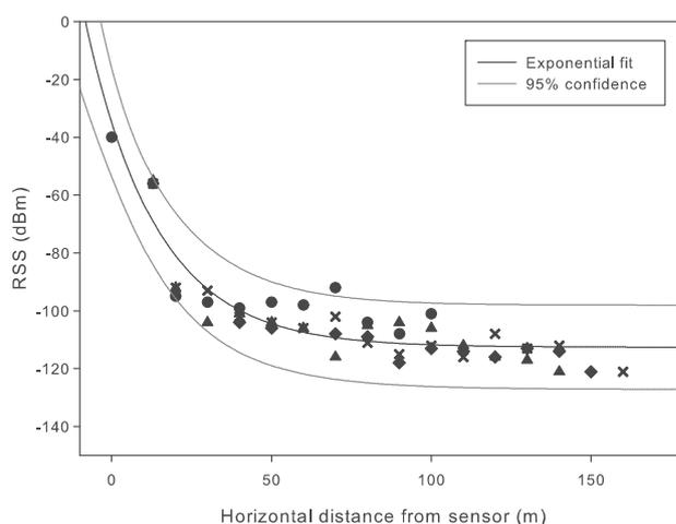
**Fig. 4.** Received signal strength (RSS) during multidirectional range tests from a sensor buried in shallow (15 cm) firn, using the WinRadio receiver. The different markers represent different radial directions as the receiver was moved away from the sensor, although the exponential fit line is based on all data ( $r_2 = 0.84$ ), with red lines denoting 95% confidence.
