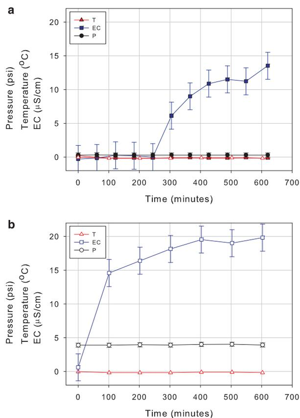
**Fig. 3.** Temperature, pressure and electrical conductivity transmitted by an ET+ sensor during meltwater percolation experiments. The dots represent hourly averages of the 30 s measurements. In the subsequent second experiment (b), snow was more tightly packed above the sensor and hence pressure readings were slightly elevated. The height of the snow did not change noticeably during the experiments
