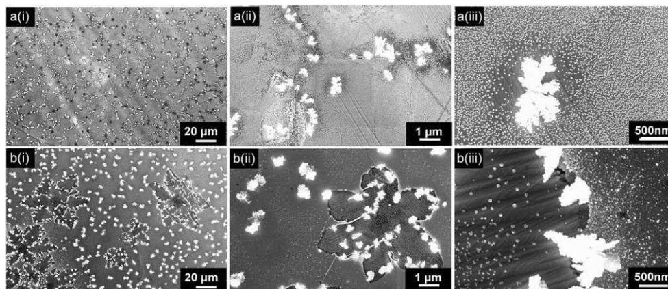
Fig. 2 SEM images of a(i–iii) full covered CVD-Gr and b(i–iii) partially covered CVD-Gr sample, after electrodeposition and electroless deposition of  $\text{AgNPs}$  (at three different magnifications). The SEM images were acquired after electrodeposition at  $0.4 \text{ V}$  for  $30 \text{ s}$  in  $0.7 \text{ mM}$  of  $\text{AgNO}_3$  in  $0.2 \text{ M}$   $\text{KNO}_3$ .
