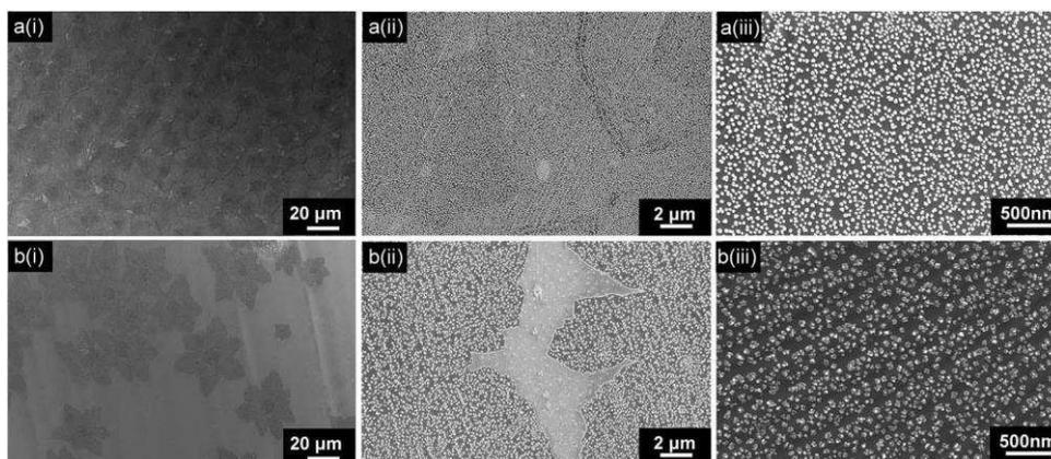
Fig. 3 SEM images of a(i–iii) full covered CVD-Gr and b(i–iii) partially covered CVD-Gr sample at three different magnifications after electro-deposition of AgNPs, whilst avoiding the electroless process. To avoid the electroless process the applied potential was adjusted to 0.46 V, and the electrochemical cell was mounted before adding the AgNO<sub>3</sub>. The working solution consisted of 0.7 mM of AgNO<sub>3</sub> in 0.2 M KNO<sub>3</sub>.
