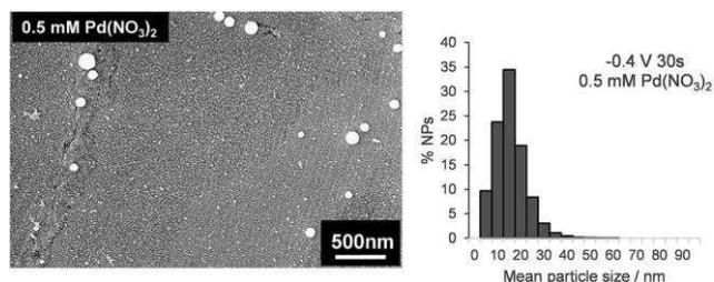
Fig. 6 SEM analysis of electrodeposition of PdNPs at a CVD-Gr electrode obtained by stepping the voltage 0.0 V to 0.4 V for 30 s, in a solution containing 0.5 mM Pd(NO<sub>3</sub>)<sub>2</sub> in 0.2 M KNO<sub>3</sub>.
