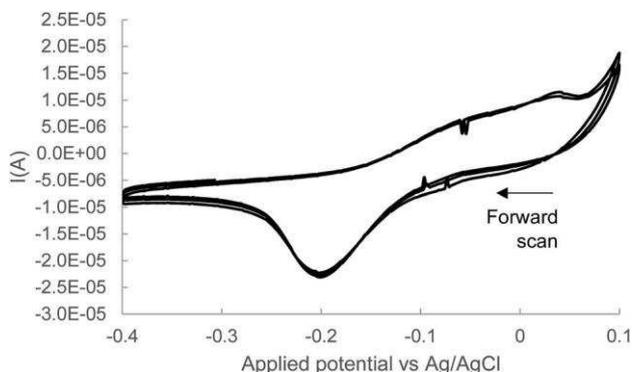
Fig. 1 Cyclic voltammogram at  $0.1 \text{ V s}^{-1}$  for the reduction of  $0.7 \text{ mM}$   $\text{AgNO}_3$  in  $0.2 \text{ M}$   $\text{KNO}_3$  using CVD-Gr as working electrode, with electrode surface area  $0.05 \text{ cm}^2$ . The spikes between  $0.1$  and  $0.05 \text{ V}$  are acquisition artefacts.
