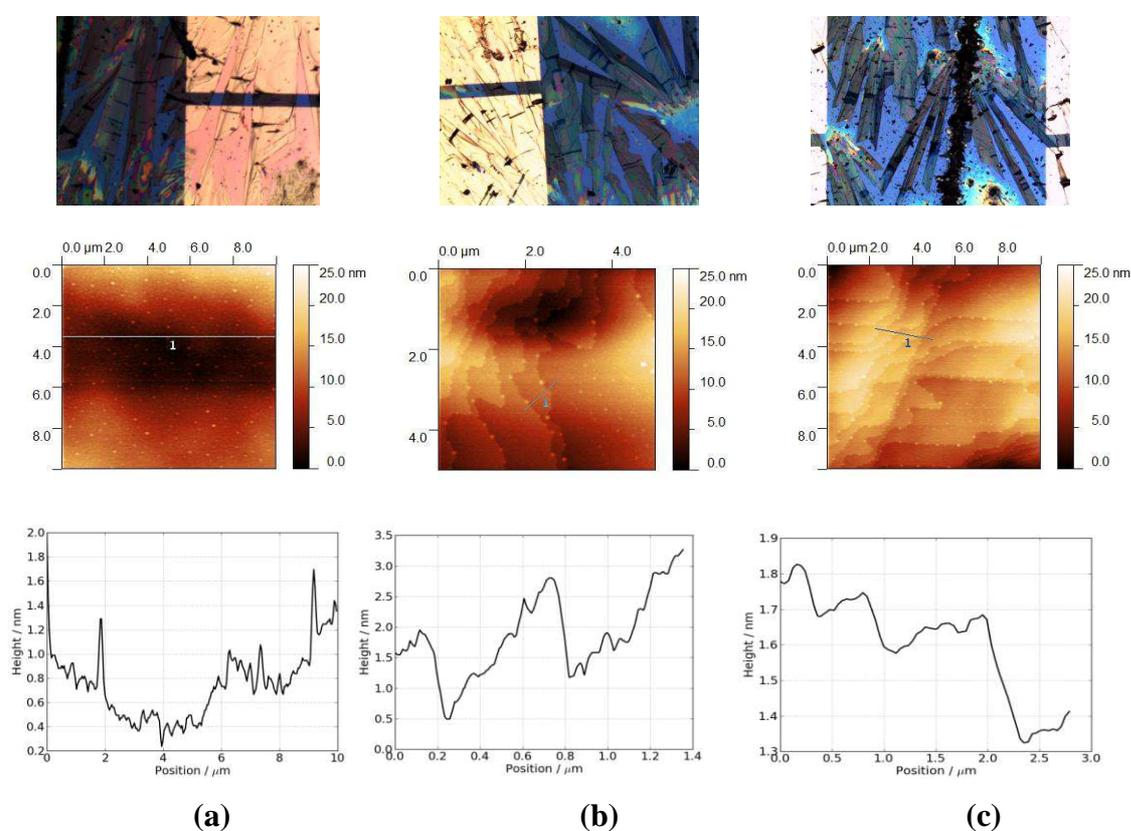
**Figure 2.** TIPS-pentacene as a function of anisole/decane wt-% ratio. (a) pure anisole, (b) anisole/decane 96/4 wt-%, (c) anisole/decane 90/10 wt-%. Top: Optical image with the golden areas showing vacuum-deposited gold electrodes, channel length 60 μm. Middle: AFM images for which the numbered sections are shown in the corresponding bottom panel.
