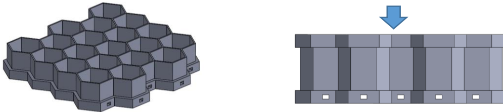
192 Figure 4. a) sectioned view of the honeycomb part, b) indication of load direction on part
