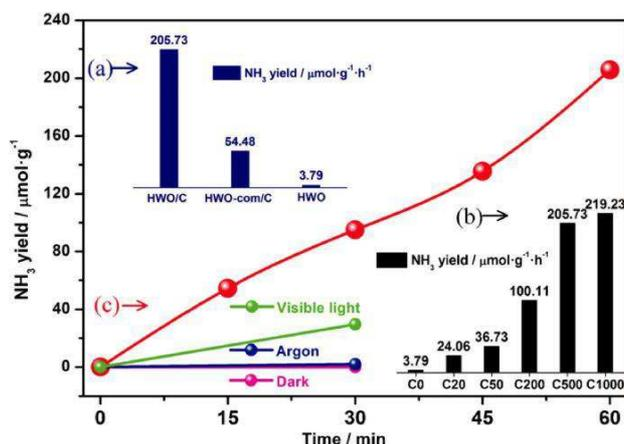
Figure 2. Photocatalytic  $\text{N}_2$  fixation rate. (a) Photocatalytic  $\text{N}_2$  fixation rates of different samples. (b) Photocatalytic  $\text{N}_2$  fixation rates of HWO/C-X samples. (c) Photocatalytic  $\text{N}_2$  fixation rates of HWO/C500 with time under UV/Vis light (red), dark (pink), visible light (green) and argon atmosphere (blue), respectively.
