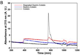
Figure 2. SEC chromatograms of colistin (black), dextrin—colistin conjugate (blue), and α-amylase-treated (48 h at 37 °C) dextrin—colistin conjugate (red) by (A) RI detection and (B) UV detection ( $\lambda$  = 215 nm). Collected fractions are shown in orange.
