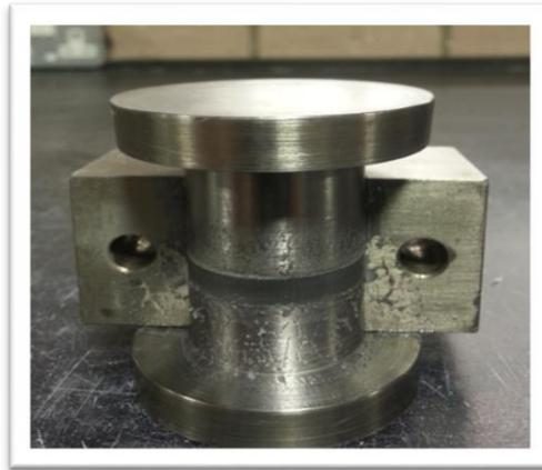
**Figure 5-2 Separate block die used in this study.**
