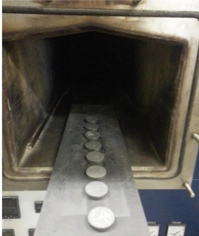
**Figure 5-5 Samples after sintering.**
