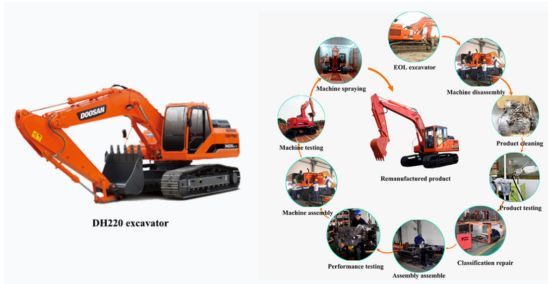
Fig. 3 Excavator of model DH220 and remanufacturing process of excavator
