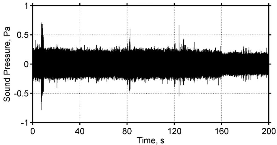
Figure 6. Resulting acoustic waveform from the start of the loading to peak load
