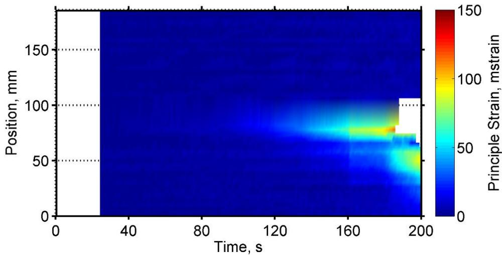
Figure 4. Principle strain along a vertical line placed at LHS high strain regions during the load regime
