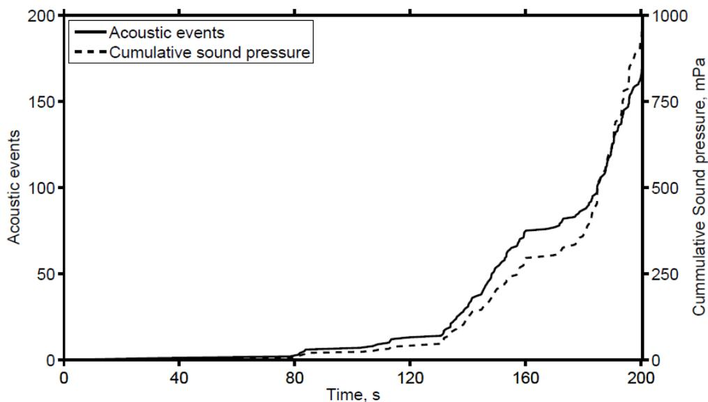
Figure 8. Rate of acoustic events and the corresponding cumulative pressure level
