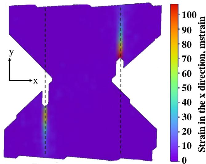
Figure 3. Strain in the x direction at peak load
