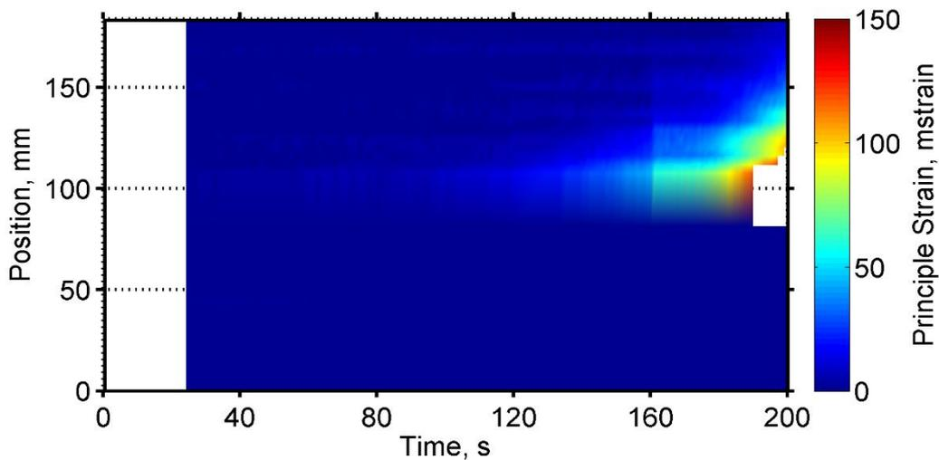
Figure 5. Principle strain along a vertical line placed at RHS high strain regions during the load regime
