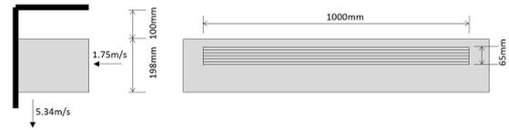
Figure 3: details of the air curtain
