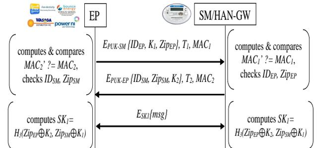
Fig. 3: Authentication between the EP and the SM.
