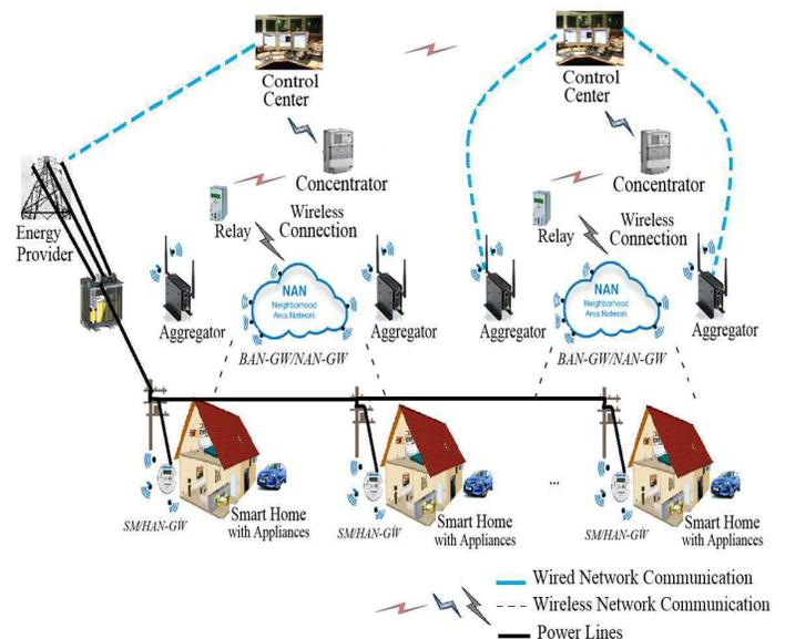
Fig. 1: Overall architecture of the smart grid system.
