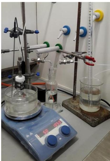
*Figure 2.5. Photograph of the reaction set-up used for the volumetric quantification of hydrous hydrazine decomposition.*
