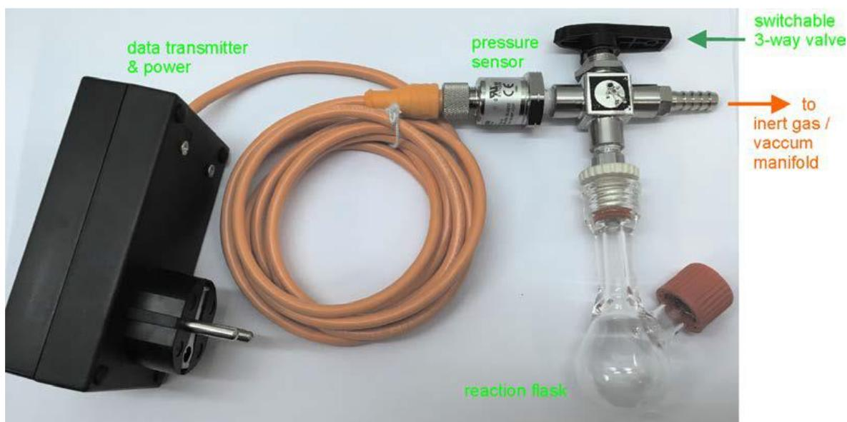
Figure 2.6. Photograph of the reaction set-up used for the volumetric quantification of hydrous hydrazine decomposition used for test homogeneous catalysts.
