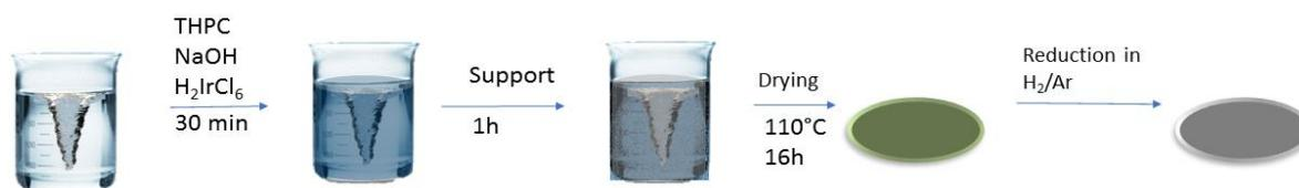
Figure 2.2. Schematic representation of sol-immobilisation with THPC for Ir catalysts used in this thesis.
