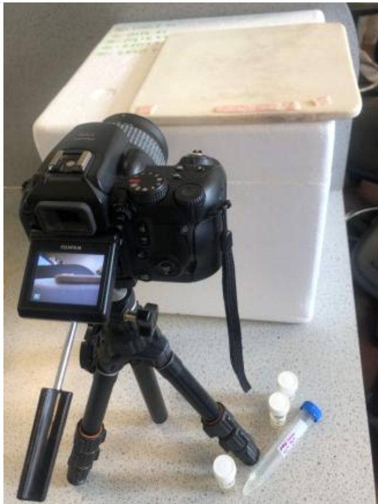
Figure 7-5 Contact angle camera set up for capturing side-on images of 50 \mu\text{L} quots of formulation on porcine skin.
