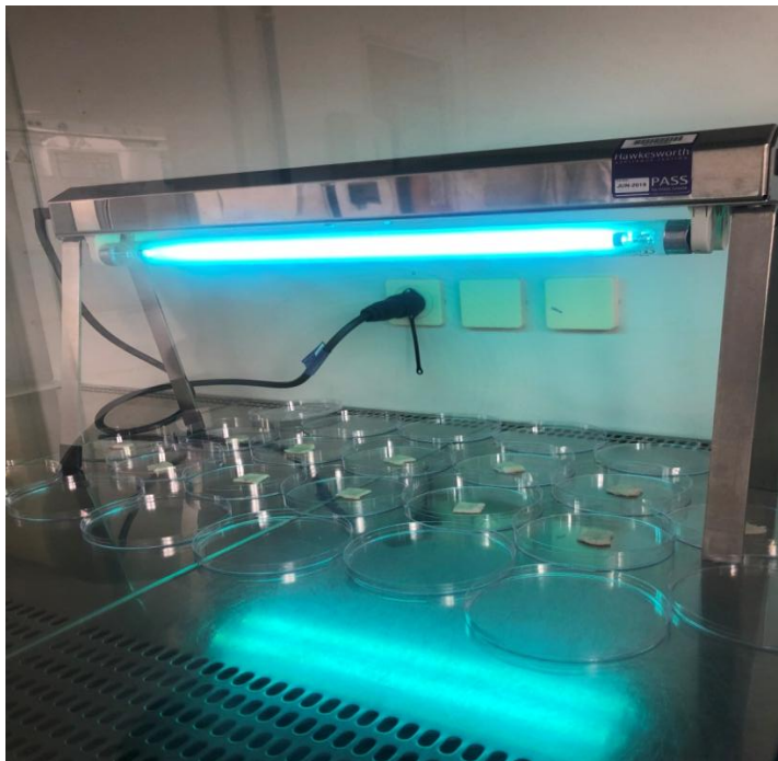
Figure 9-1 Sterilisation of porcine skin samples by treatment with UV lamp to ensure skin microbes had been eradicated prior to the inoculating with bacteria.
