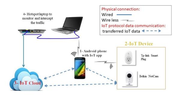
Figure 3.1: IoT Compliance Testbed
