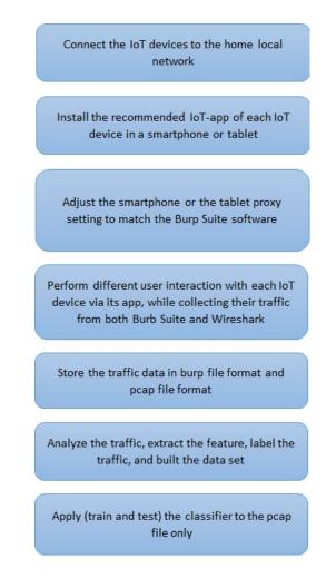
Figure 5.2: Overview of the steps used to collect the encrypted TLS traffic and the encrypted one of the IoT device to establish the ground truth of the IoT-app PIT.
