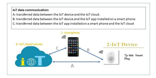
Figure 3.2: Methods of IoT communication with its cloud to transfer data
