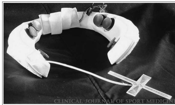
Figure 2-1: HIT player unit, consisting of 6 accelerometers in spring-loaded holders, frequency modulation antenna, and rechargeable battery pack.[ 59]
