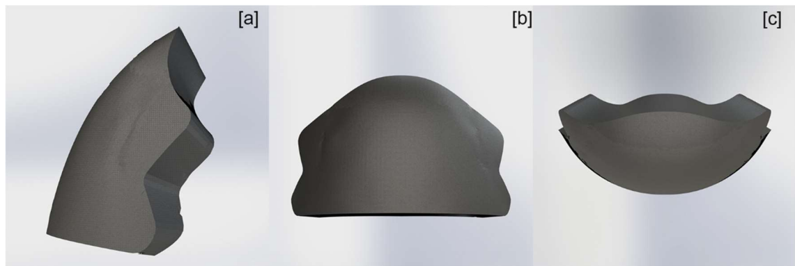
Figure 7-1: Render of the Front pad of a Riddell Speed helmet (2016) isolated from CAD geometry, side view [a], front view [b] and top view [c].
