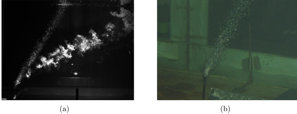
Figure 5.28: Images of PIV experiments showing the bubble column for 0.10m/s crossflow and 0.5l/min bubble flow rate.
