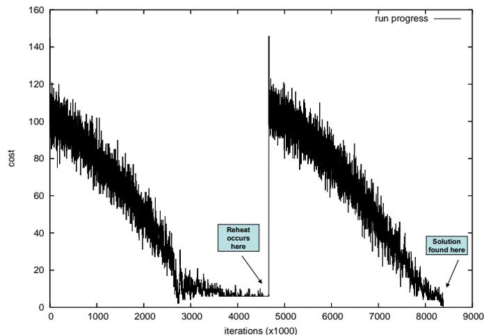
**Figure 3.** A typical run of the SA algorithm using an order-4 instance taken from *The Independent* on Saturday, June 18<sup>th</sup> 2005. This run required one reheat and took approximately 8 seconds to find a solution.
