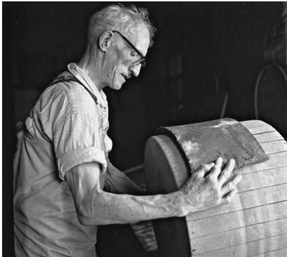
Fig. 5. Mr. Fred Boulton rolling a strip of side-marl onto a wooden drum. Photographed at the *Burgess and Leigh* Factory, Middleport 1964. (Photo by and reproduced courtesy of Mr. Donald Morris).
