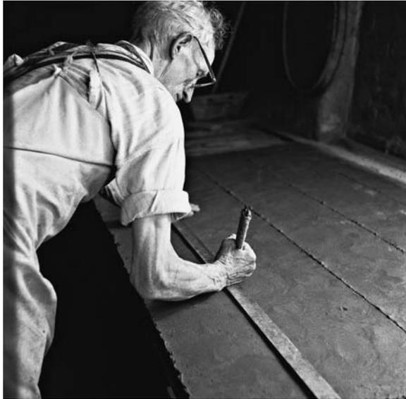
Fig. 4. Mr. Fred Boulton using a wooden straight edge — “rule” — and blade to cut strips of side-marl to the appropriate width ready to be rolled onto a wooden drum. Photographed at the *Burgess and Leigh* Factory, Middleport 1964. (Photo by and reproduced courtesy of Mr. Donald Morris).
