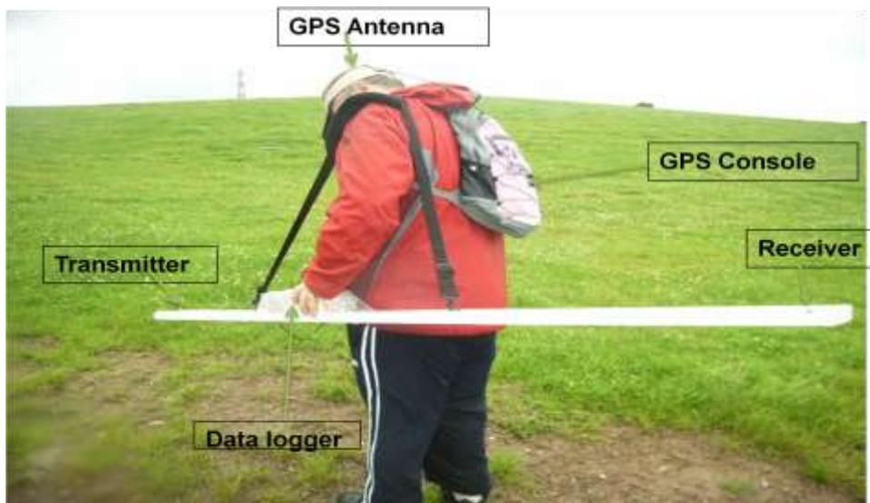
Figure 6: Showing the setup of GEM-2 and the GPS device
