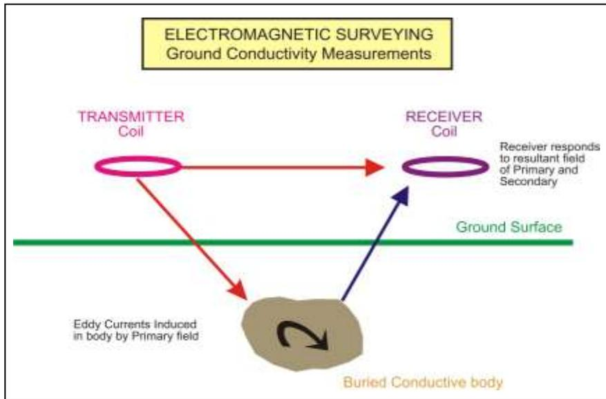
Figure 5: The schematic diagram showing the principle of the EM technique for site investigation
