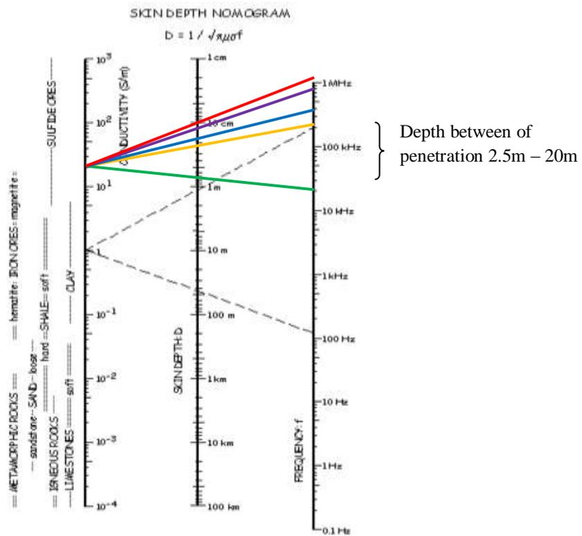
Figure 8: ‘Skin Depth Nomogram’ diagram is used to determine depth of layers
