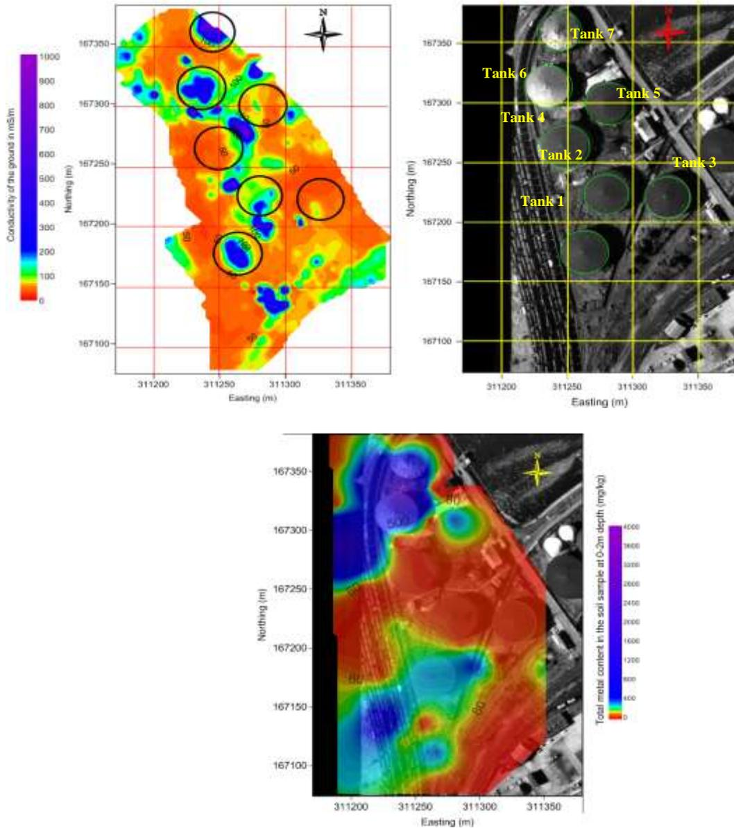
Figure 9: Showing interaction between the conductivity of the material and the TPHs distribution.
