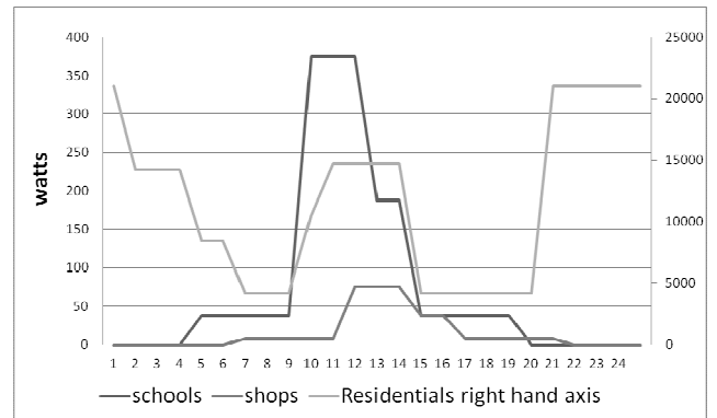
Figure 4: DHW heat demand of three types of properties (Residential street with the right hand Y Axis, School and shops with the left hand Y Axis)
