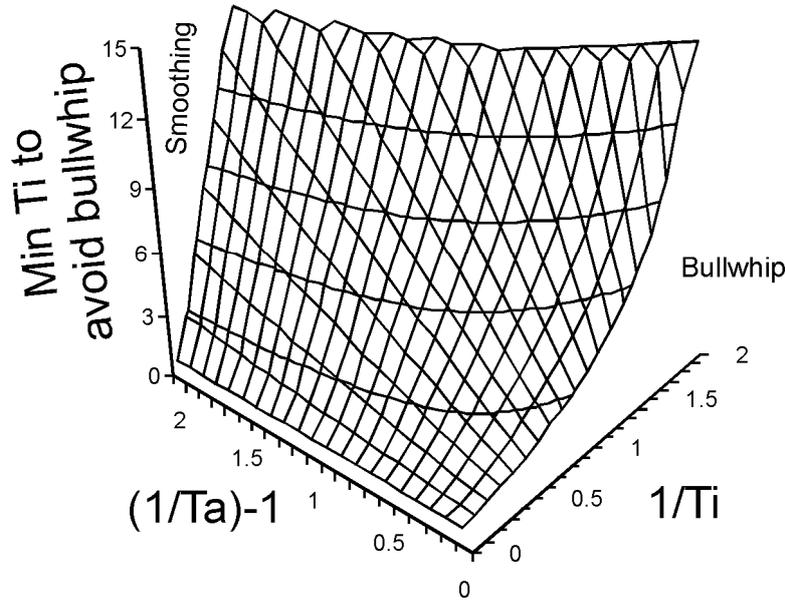
**Figure 3. The Bullwhip boundary for DE-APIOBPCS**
