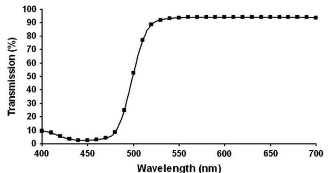
**Figure 2.** Light transmission spectrum of riboflavin solution.
