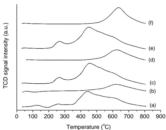
**Fig. 2** TPR profiles for Au/C catalysts subject to reduction and oxidation cycles, (a) fresh catalyst, (b) reduced catalyst, (c) first catalyst oxidation, (d) second catalyst reduction, (e) second catalyst oxidation, (f) third catalyst reduction
