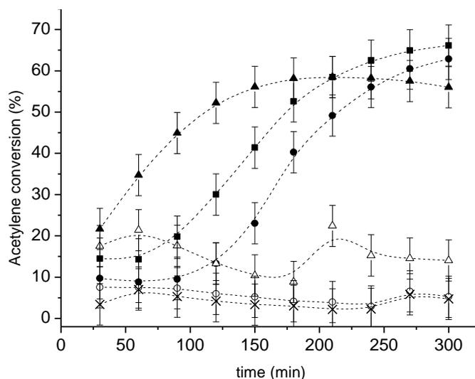
**Fig. 1** Acetylene conversion over Au/C (1% wt) catalysts subject to reduction and oxidation cycles, (■) fresh catalyst, (○) reduced catalyst, (●) first catalyst oxidation, (Δ) second catalyst reduction, (▲) second catalyst oxidation, (x) third catalyst reduction.
