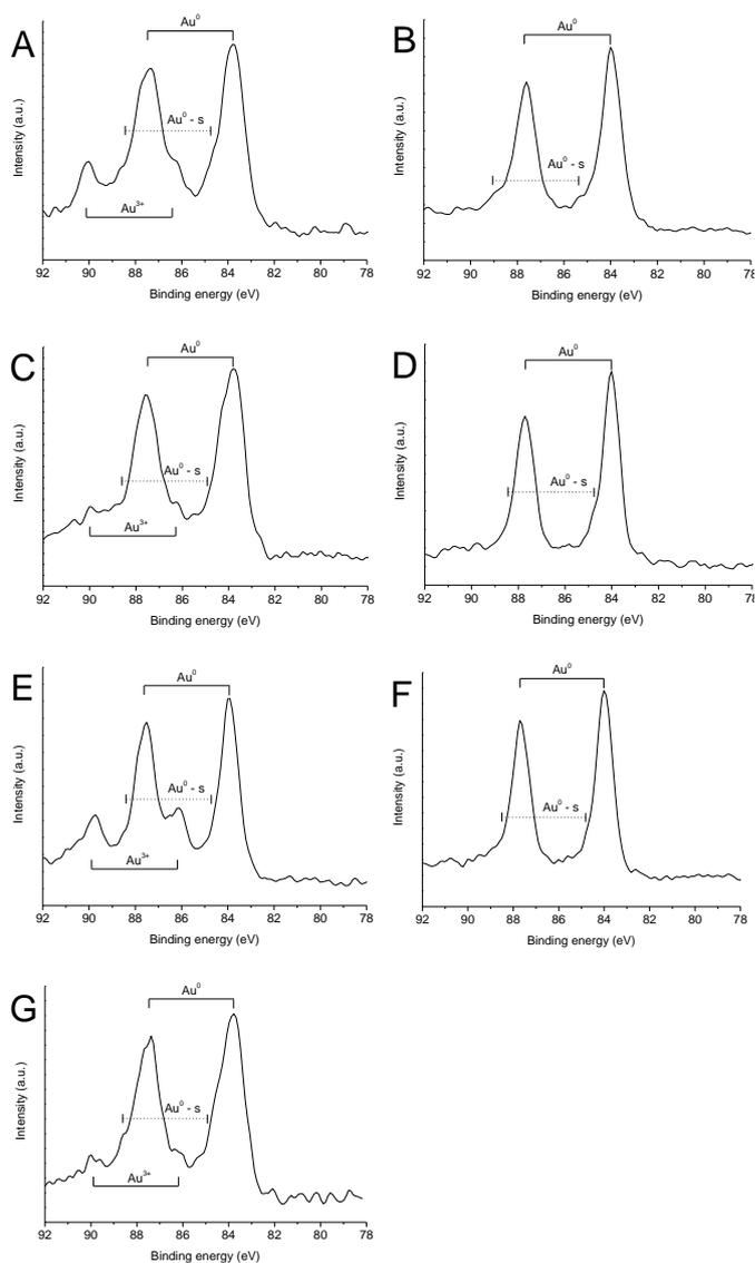
**Fig. 4** XPS profiles for Au/C catalysts subject to reduction and oxidation cycles, (A) fresh catalyst, (B) reduced catalyst, (C) first catalyst oxidation, (D) second catalyst reduction, (E) second catalyst oxidation, (F) third catalyst reduction and (G) third catalyst oxidation.
