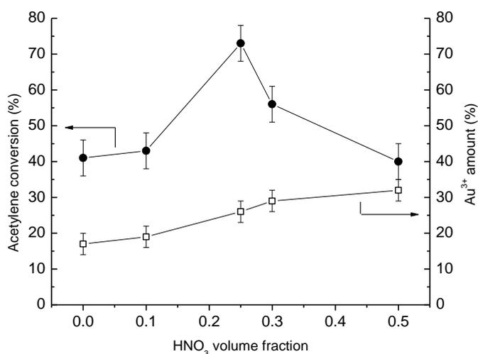
**Fig. 3** Conversion (●) after 5 h and Au<sup>3+</sup> (□) amount for Au/C catalysts containing different amount of Au<sup>3+</sup>. The catalysts were obtained from impregnation using solutions containing different HNO<sub>3</sub> volume fraction in the HCl/HNO<sub>3</sub> mixture.
