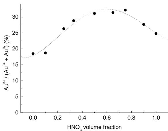
**Figure 9.** TPR intensities for the reduction of Au<sup>3+</sup> species for Au/C catalysts prepared using different HNO<sub>3</sub> volume fraction in the HCl:HNO<sub>3</sub> solvent mixture. All catalysts were dried at 140 °C.
