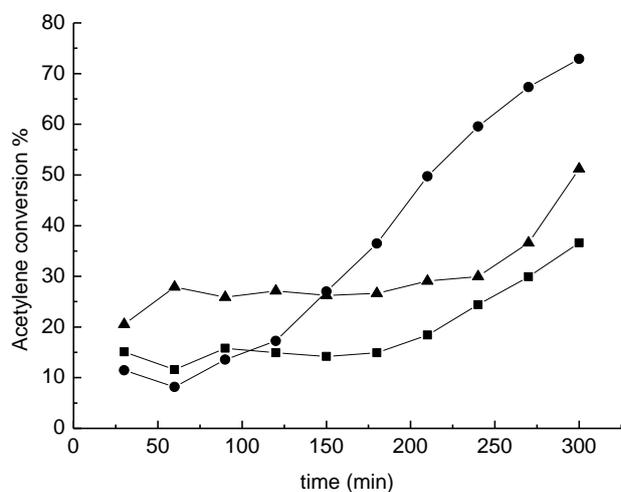
**Fig. 1.** Acetylene conversion by using catalysts impregnated in *aqua regia*, drying the catalysts at temperatures of: (■) 110, (●) 140 and (▲) 180 °C.
