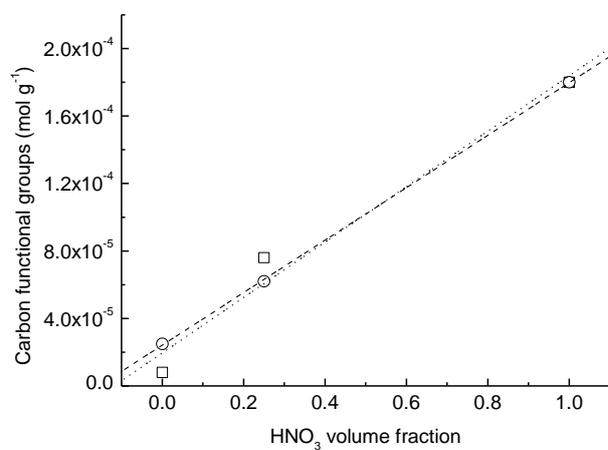
**Fig. 11.** Oxygenated carbon functional groups (carboxylic/lactones) induced by the presence of HNO<sub>3</sub> in the preparation mixture for HCl, aqua regia, and HNO<sub>3</sub>, (○) and (- -) Au/C catalysts, (□) and (··) Au/C catalysts from acid pre-treated carbons.
