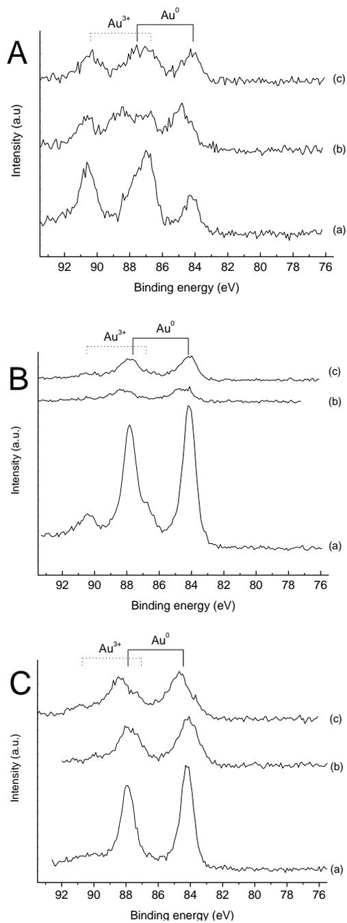
**Figure 5.** XPS spectra of Au/C carbon prepared accordingly to different solvent and drying temperature: A: (a) HCl, (b) HNO<sub>3</sub> and (c) *aqua regia* for catalysts dried at 110 °C; B: (a) HCl, (b) HNO<sub>3</sub>, and (c) *aqua regia* for catalysts dried at 140 °C; C: (a) HCl, (b) HNO<sub>3</sub> and (c) *aqua regia* for catalysts dried at 180 °C.
