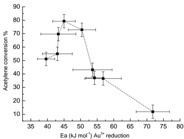
**Figure 12.** Maximum acetylene conversion (after 5h) versus activation energies for the reduction of Au<sup>3+</sup> in hydrogen.
