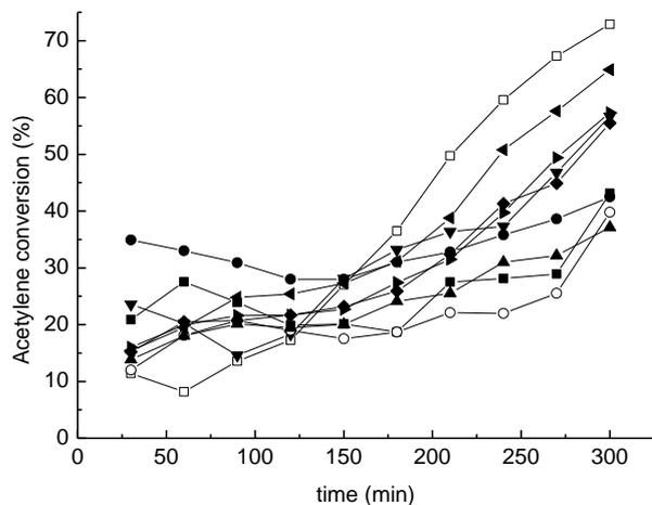
**Figure 6.** acetylene conversion over Au/C catalysts dried at 140 °C using different HNO<sub>3</sub> volume fraction in the HCl:HNO<sub>3</sub> preparation mixture: (■) 0, (●) 0.1, (□) 0.25, (▼) 0.33, (○) 0.5, (◄) 0.65, (►) 0.75, (◆) 0.9 and (▲) 1 HNO<sub>3</sub> volume fraction.
