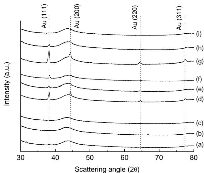
**Figure 4.** XRD patterns of Au/C carbon prepared accordingly to different solvent and drying temperature: (a) HCl, (b) HNO<sub>3</sub> and (c) *aqua regia* for catalysts dried at 110 °C; (d) HCl, (e) HNO<sub>3</sub>, and (f) *aqua regia* for catalysts dried at 140 °C; (g) HCl, (h) HNO<sub>3</sub> and (i) *aqua regia* for catalysts dried at 180 °C.
