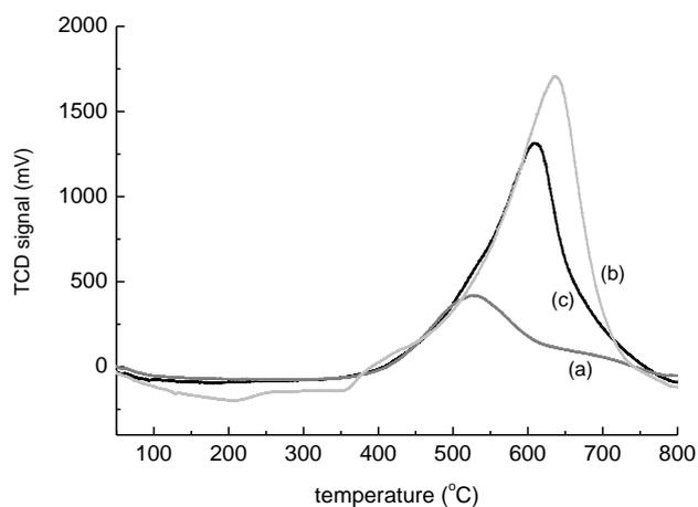
**Figure 6.** TPR profiles of carbon support Norit ROX 0.8 dried at 140 °C prepared via impregnation using: (a) HCl, (b) HNO<sub>3</sub>, and (c) *aqua regia* as solvent.
