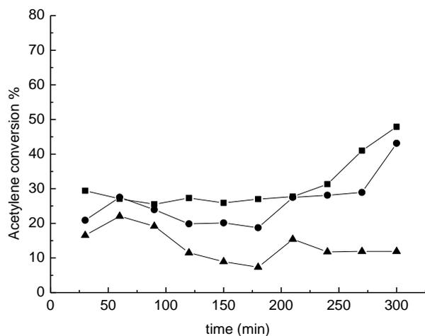
**Fig. 3.** Acetylene conversion by using catalysts impregnated in HCl drying the catalysts at different temperatures of: (■) 110, (●) 140 and (▲) 180 °C.
