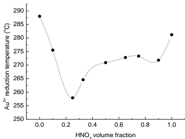
**Figure 10.** Au<sup>3+</sup> reduction temperature from temperature programmed reduction in presence of H<sub>2</sub> for Au/C catalysts prepared using different HNO<sub>3</sub> volume fractions in the HCl:HNO<sub>3</sub> solvent mixture. All catalysts were dried at 140 °C.
