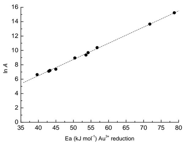
**Figure 13.** Compensation plot for the reduction of Au<sup>3+</sup> over Au/C using H<sub>2</sub>, for catalysts prepared using HCl, HNO<sub>3</sub> and *aqua regia*, dried at 110, 140 and 180 °C.
