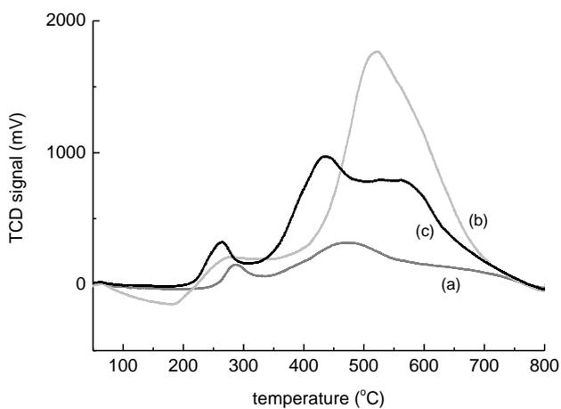
**Figure 5.** TPR profiles of Au/C catalysts dried at 140 °C prepared via impregnation using: (a) HCl, (b) HNO<sub>3</sub>, and (c) *aqua regia* as solvent.
