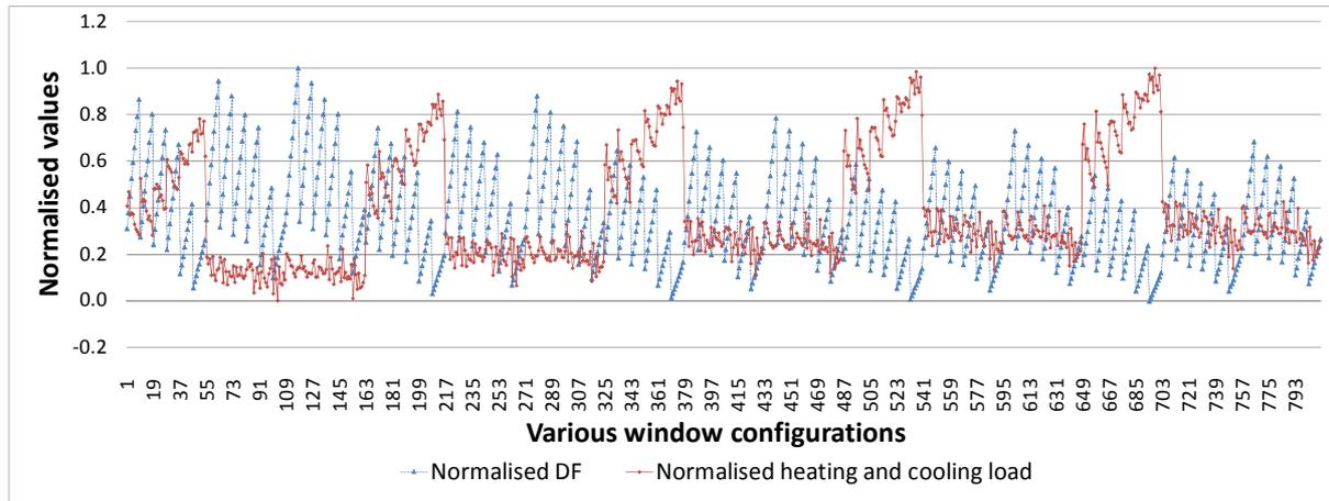
Figure 5: Comparison of normalised DF and cooling/heating loads for variable window configurations.
