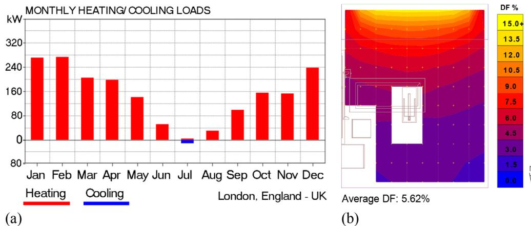
(a) Figure 7: Monthly cooling and heating load distribution (a) and average daylight factor of the room (b) for optimal solution.
