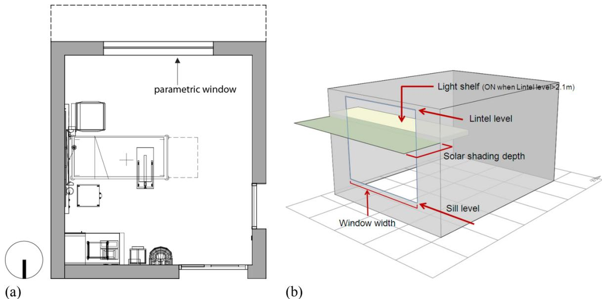
Figure 1: (a) The plan of the patient room, and (b) The parametric window model illustrating the decision variables.
