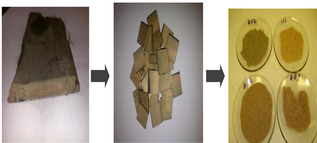
**Figure 4.5 Sample preparation stages from wood section into chips then sawdust**
