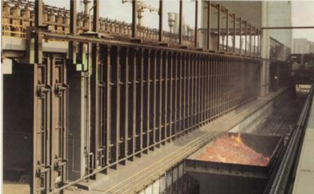
**Figure 4.2 Incandescent coke pushed from coke on a quenching car, ready to be taken to the quenching tower [94]**
