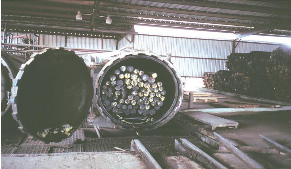
**Figure 2.2 Convectional pressure cylinder and locking doors with loaded wood for preservative treatment [28]**
