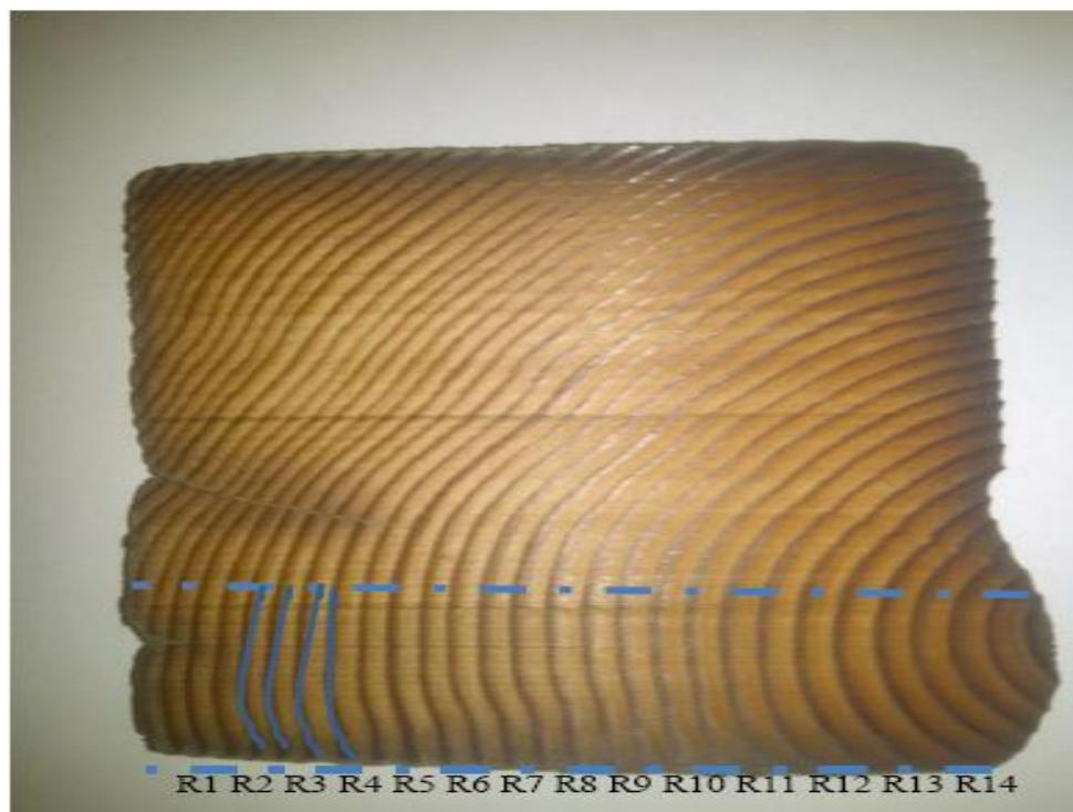
**Figure 4.7 Edge assessment with multiple growth rings cut according to the indicated marks and labelled samples accordingly**
