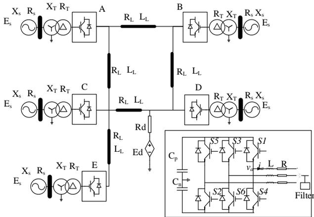
Fig.10 Topology of DC grid with five terminals
