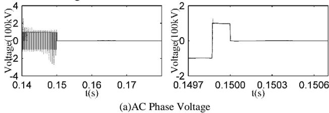
Fig. 18 Short-circuit of converter bridge
