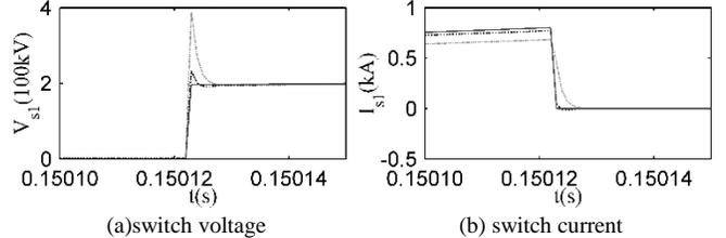
Fig.13 Normal operation of switch  $S_1$  of VSC
