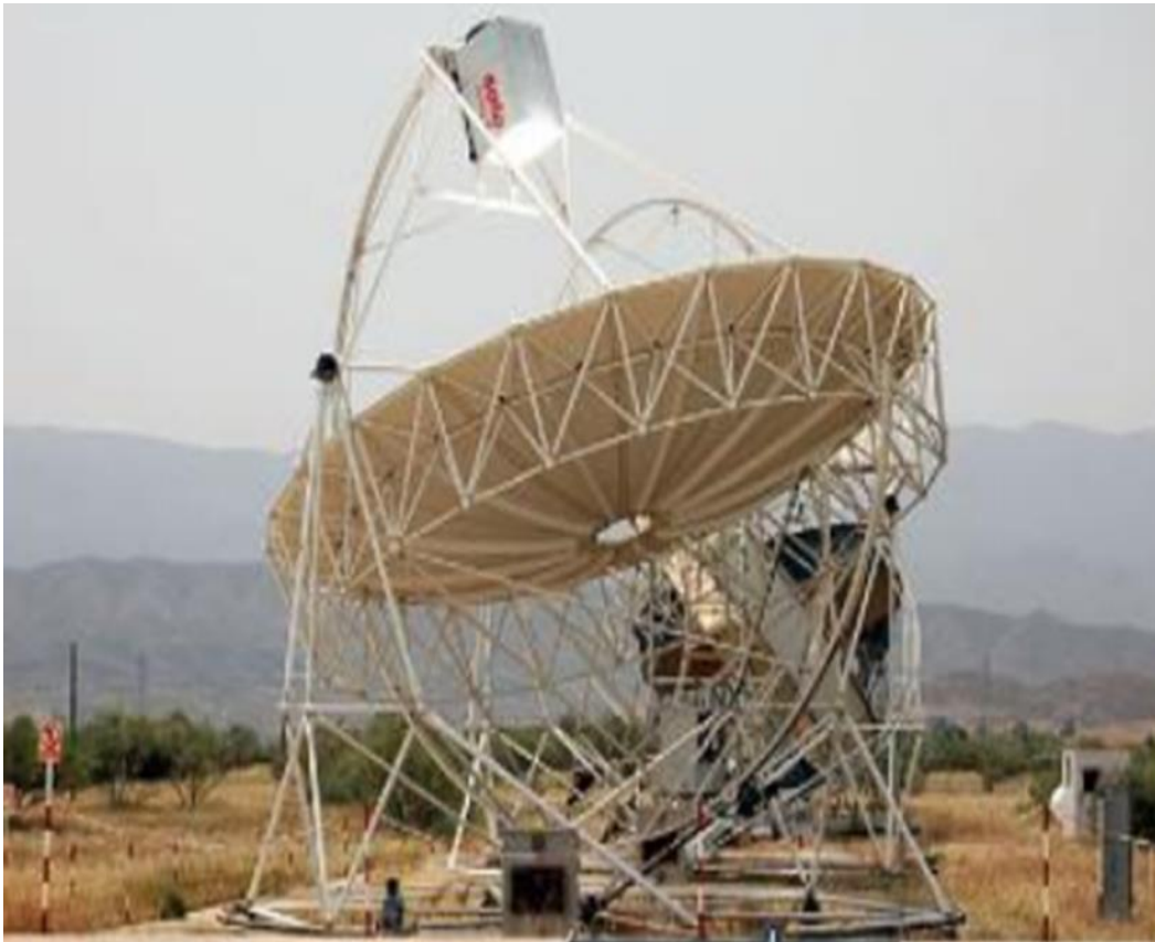
Figure 2.6 A dish collector and its mounted receiver (Camacho et al., 2012).
