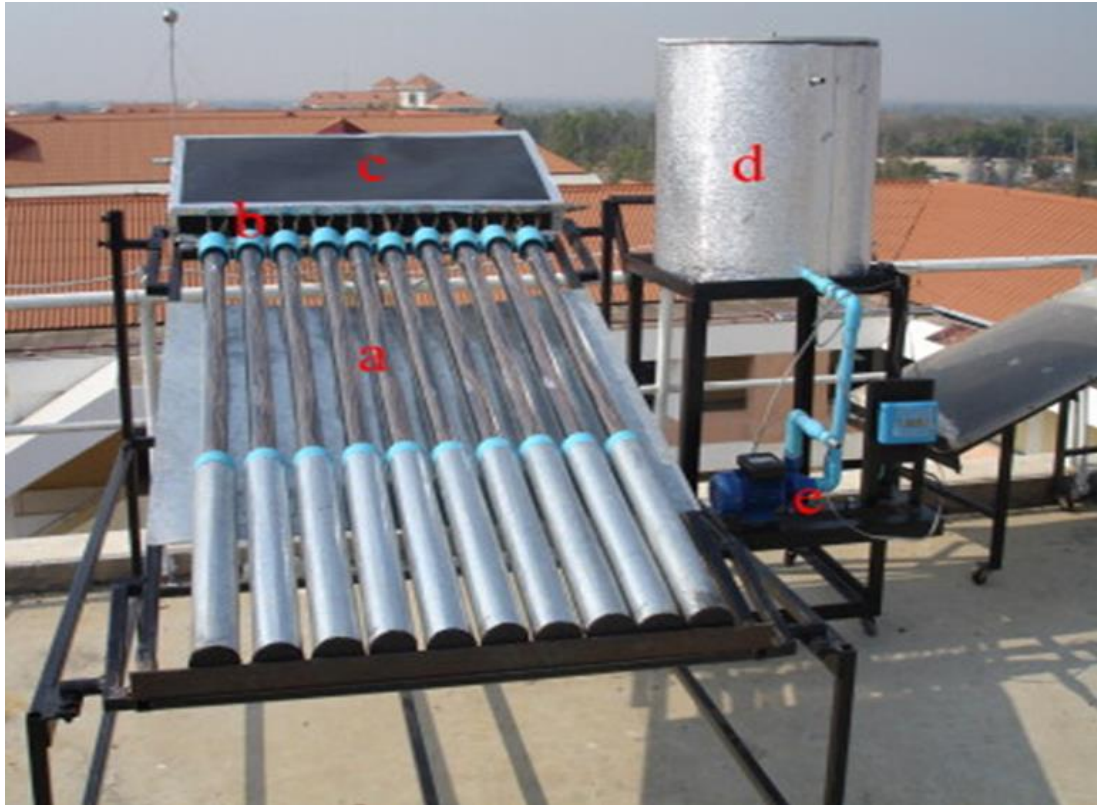
Figure 2.8 An active SWH system in closed loop (a) solar collector; (b) gap between the pipes and the tank; (c) water tank; (d) water storage tank; (e) water pump (Rittidech. et al., 2009).
