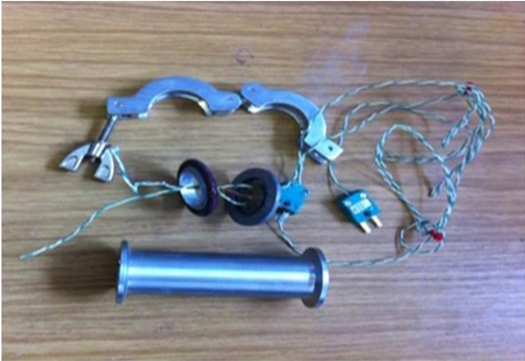
Figure 5.9 Home-made feed through using a blank cover, which can be attached to the standard KF flange.
