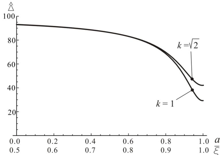
Figure 6. Impact of  $\alpha$  and  $\bar{\xi}$  on  $\hat{\Delta}$  when  $T_p = T_r = 5$ ,  $k = 1$  and  $k = \sqrt{2}$
