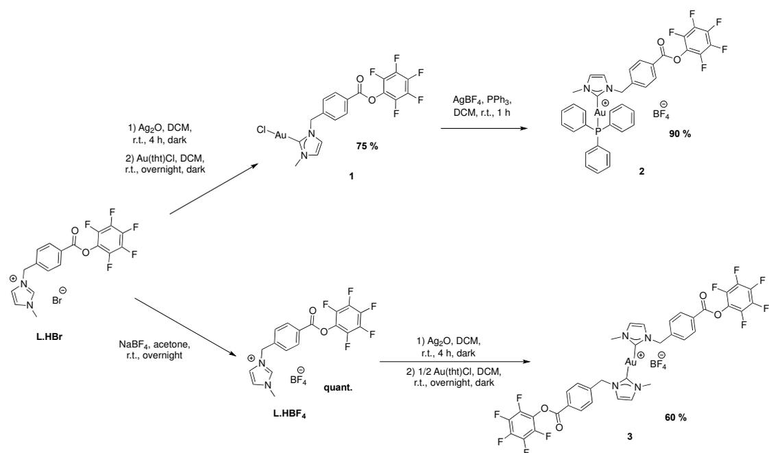
**Scheme 1:** Synthesis of the different Au(I)-NHC complexes bearing the pentafluorophenol ester moiety.
