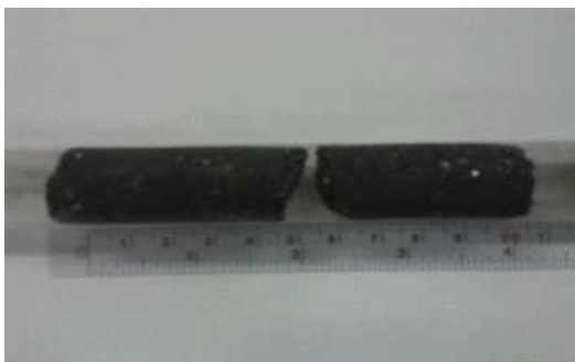
Fig. 4 Image of the cylindrical coal samples.
