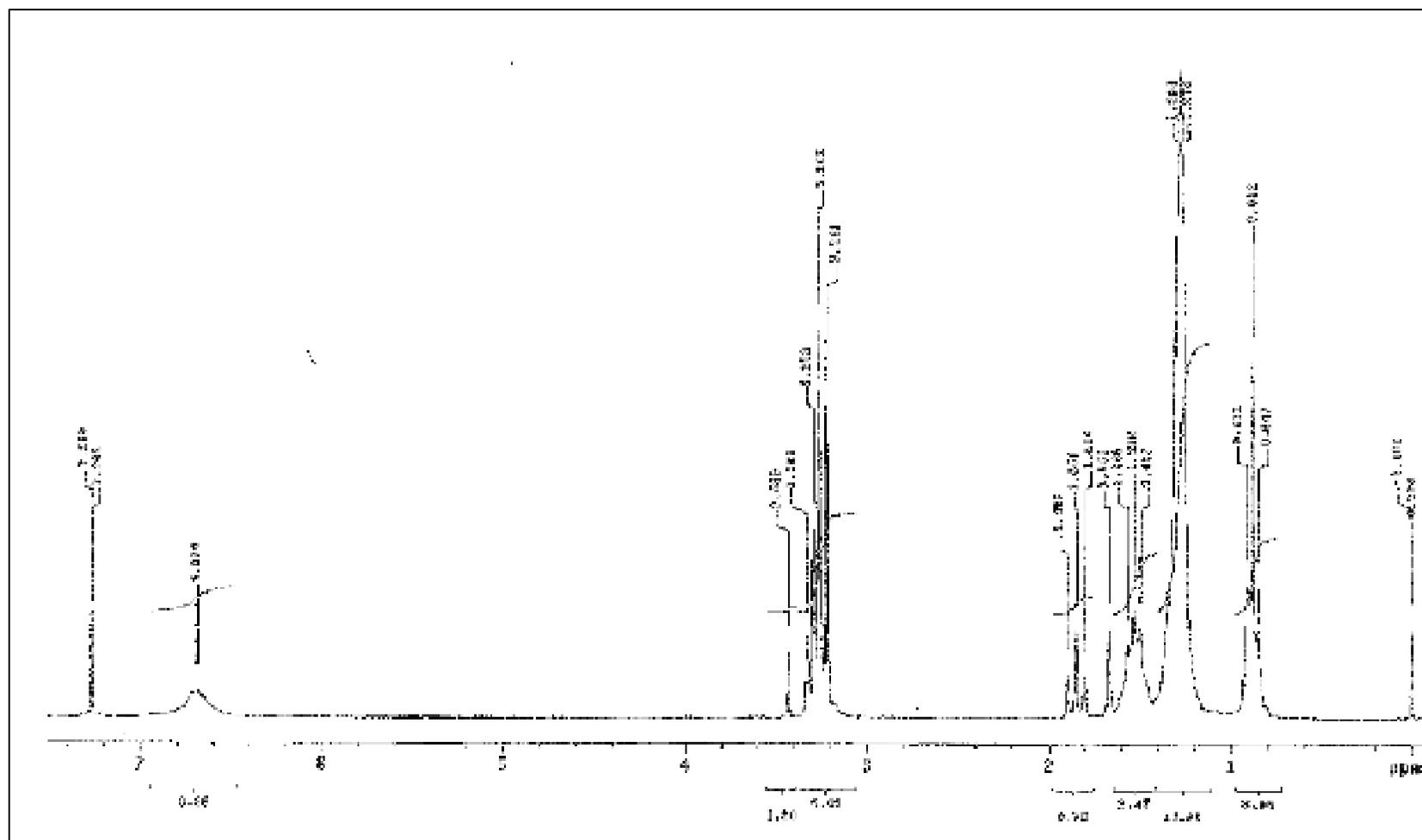
D:  $^1\text{H-NMR}$  spectrum of TGA-O in  $\text{CDCl}_3$ .
