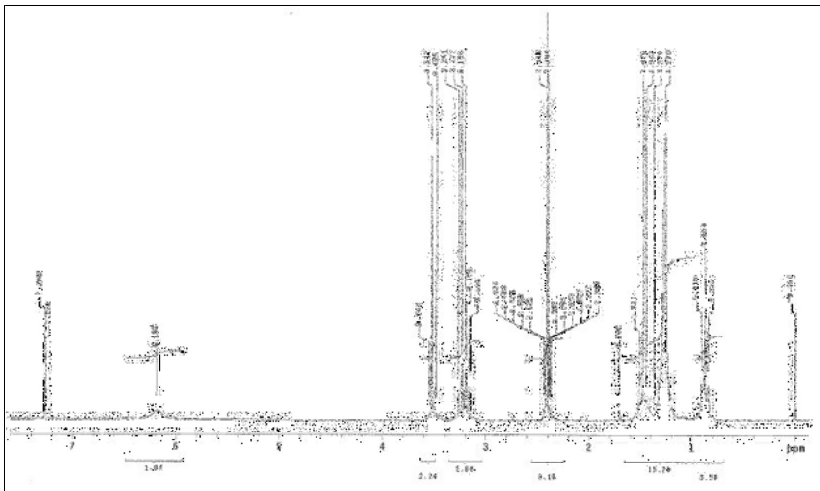
C:  $^1\text{H-NMR}$  spectrum of TGA-Octylamine-thioester in  $\text{CDCl}_3$ .
