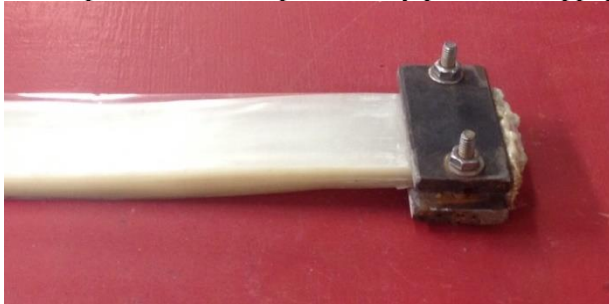
Fig. 2 SMP tendon with external anchorage for PETr prisms
