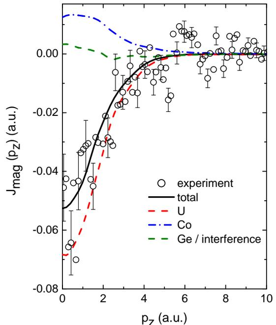
FIG. 2: Color online: Magnetic Compton profile of UCoGe along the c-axis taken at 5 T, shown with spin density predicted by KKR calculations normalized to the spin moment of  $-0.24 \pm 0.05 \mu_B$  and decomposed into the site projected profiles.
