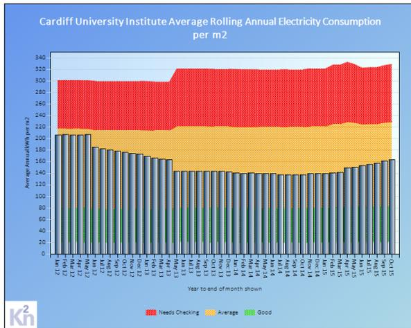
Figure 2 - Benchmark ranges for Cardiff University Annual Electricity Use per m<sup>2</sup> over last 4 years, and measured overall consumption
