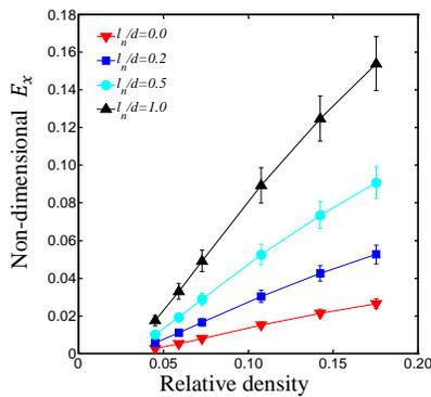
Fig3. Size-dependent effect on the relationship between the non-dimensional Young's modulus in the x direction and the relative density of stochastic fibrous materials at nano-meter scale.
