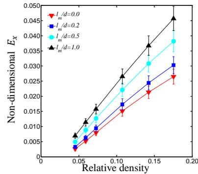
Fig2. Size-dependent effect on the relationship between the non-dimensional Young's modulus in the x direction and the relative density of stochastic fibrous materials at micro-meter scale.
