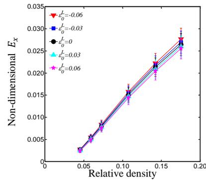
Fig4. Non-dimensional Young's modulus  $E_x$  v.s. the relative density of nano-sized stochastic fibrous networks with the presence of the effects of initial strains/stresses.
