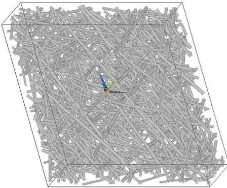
Fig1. Three-dimensional random beam model with cross-linking.
