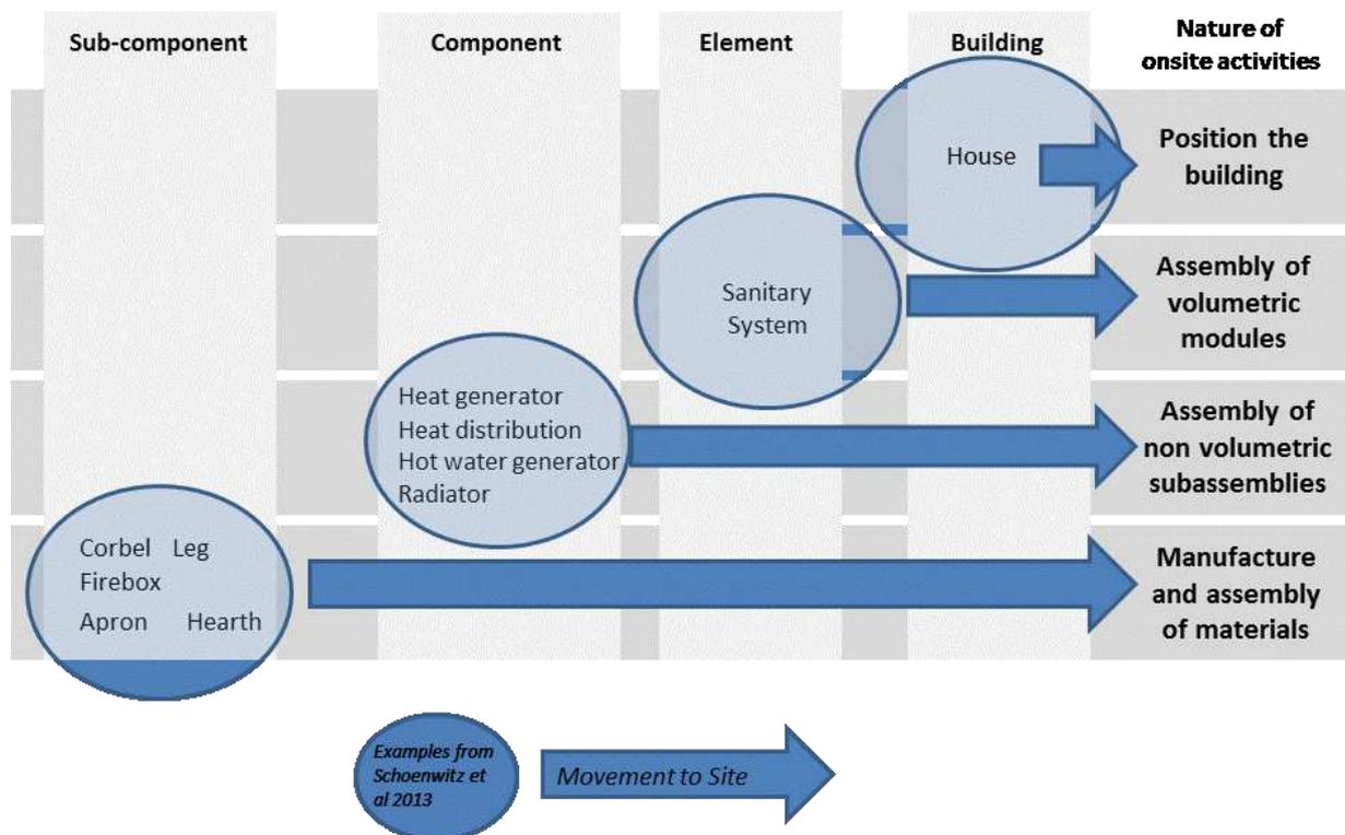
Figure 1: Potential strategies for modularization of a building at different levels
