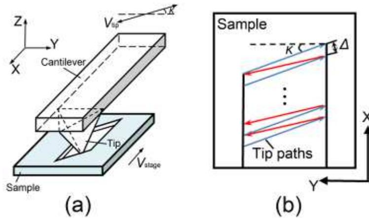
Fig. 6. (a) Schematic diagram of the nanomachining setup with an included angle and (b) the top view of the machining process.
