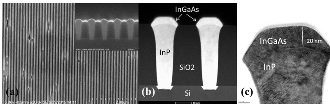
307 **Figure 8.** (a) Top-down view SEM image of InGaAs/InP fins on Si (001); Inset: SEM image
