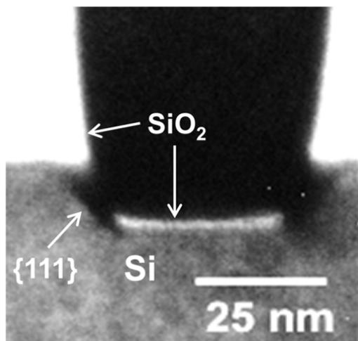
278 **Figure 1.** TEM image of a cross section of the SiO<sub>2</sub> trench with {111} Si facets exposed at
