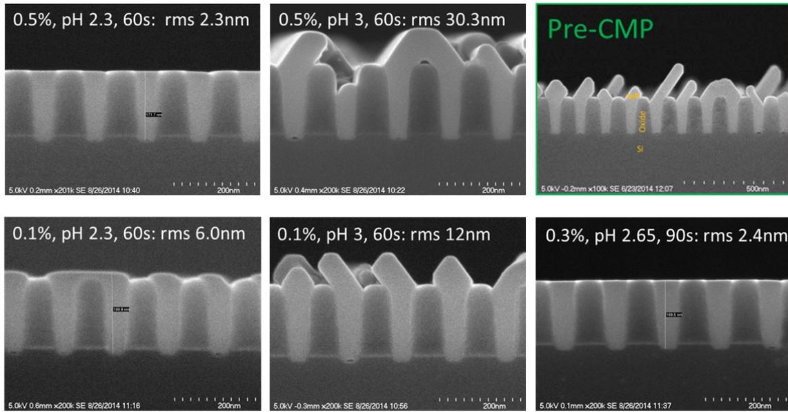
299 **Figure 6.** Cross-section SEM images of test structure post InP CMP. CMP parameters and
