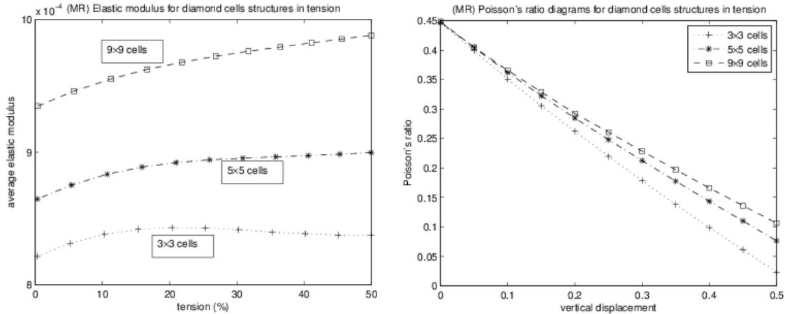
Figure 2. The non-linear elastic modulus (left) and non-linear Poisson's ratio (right) for the diamond cells of Mooney-Rivlin material with the different curves corresponding to structures with a different number of cells while the volume of elastic material is fixed.
