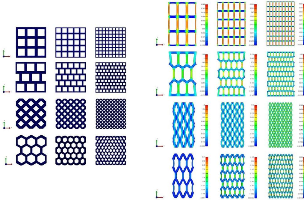
Figure 1. Undeformed model structures with different cell geometries and increasing number of cells while the volume of solid material is fixed (left) and deformed structures subject to 50% stretch in the vertical direction, showing the non-homogeneous Green-Lagrange vertical strains (right). For stacked and diamond cells, the ratio between the thickness and the length of the cell walls also remains unchanged, while for staggered and hexagonal cells, this ratio increases slightly.
